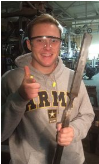
Figure A.6. Three Sheets Welded Together and Attached to Temporary Steel Handle.
