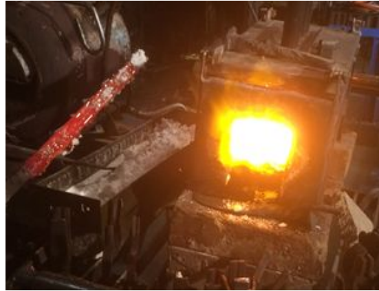
Figure 5.11. Adding Flux to the Hot Metal.
