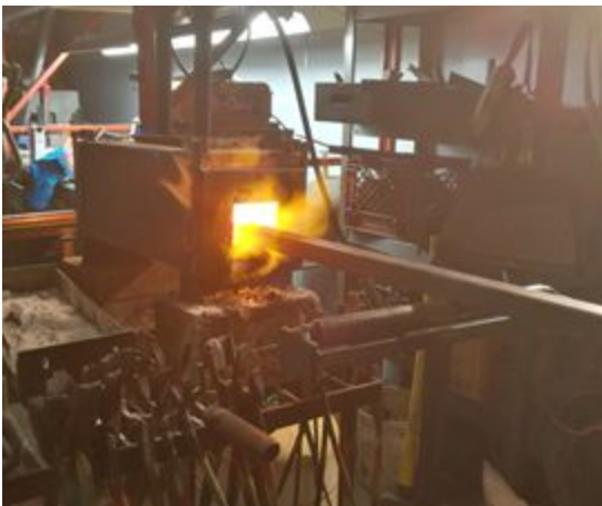
Figure A.7. Propane Furnace.
