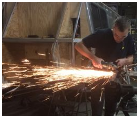
Figure A.5. Hand Grinding of The Sheets.
