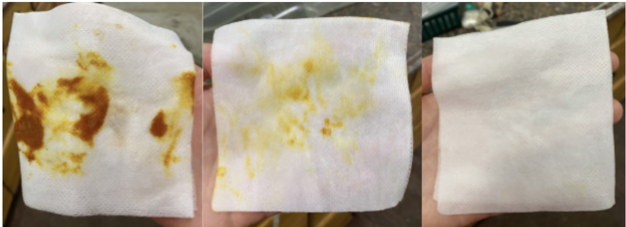
Figure 4: Progression of the coloration of 70% isopropyl alcohol wipes during sterilization method #1
