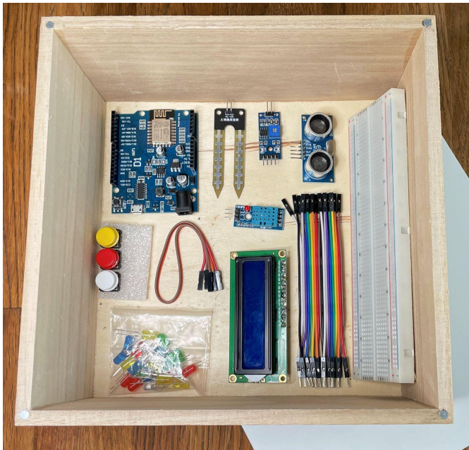
Figure 6. Makerspace Box. Mr. Köppel currently has these electronics boxes with an arduino, moisture sensor, ultrasonic sensor, temperature and air humidity sensor, digital display, breadboard, cables, knobs, and LEDs.
