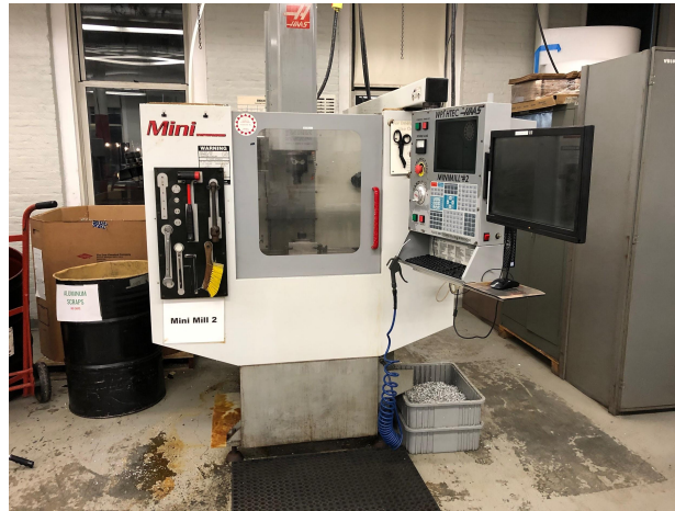
Figure 47: HAAS minimill used to manufacturer gearbox components
