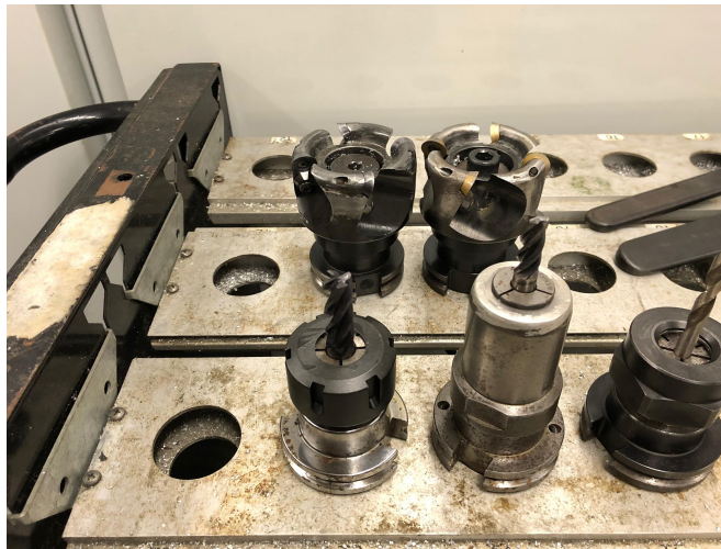
Figure 46: Tools used in minimill (3" Facemill & 3/8th Endmill)
