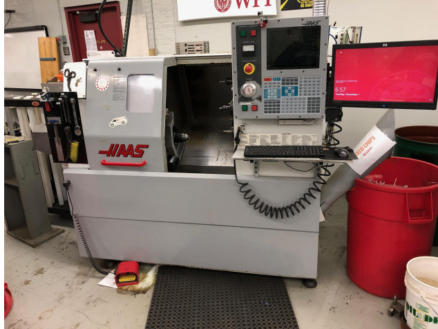
Figure 42: HAAS st-10 Lathe used to manufacture wheel
