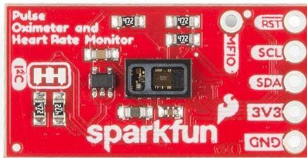
Figure 12: SparkFun Pulse Oximeter and Heart Rate Sensor - MAX30101 & MAX32664 Top View [41]
