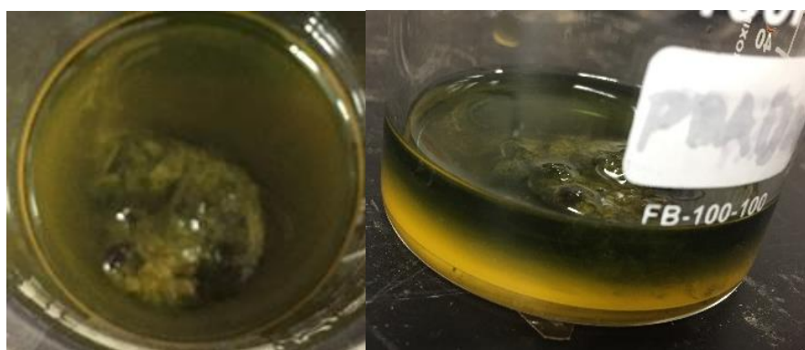
Figure 33. PSS/MA crosslinked PEC: degradation in 5 M sulfuric acid
