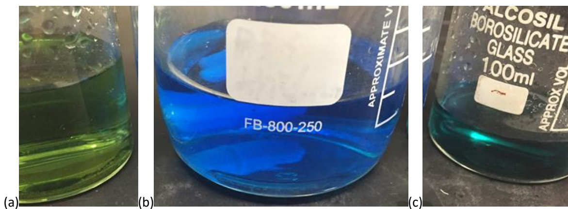
Figure 35. Solutions after complete charge (a) Cathode V^{5+} (b) Pre-charge V^{4+} (c) Anode V^{2+}
