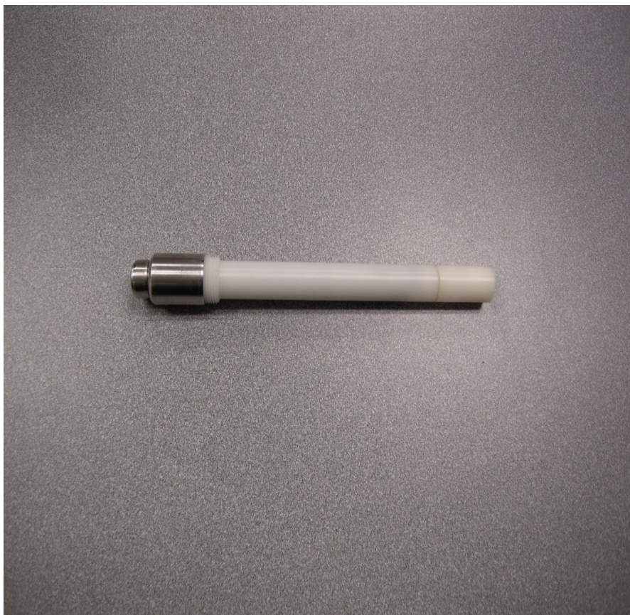
Figure 4: Fully assembled Philips body electrode
