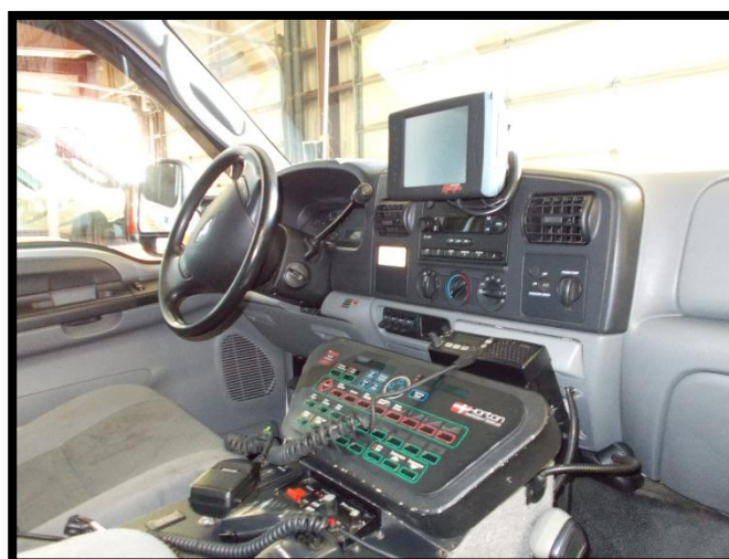
Figure 7: The communication system in an ambulance owned by UMass hospital, Worcester
