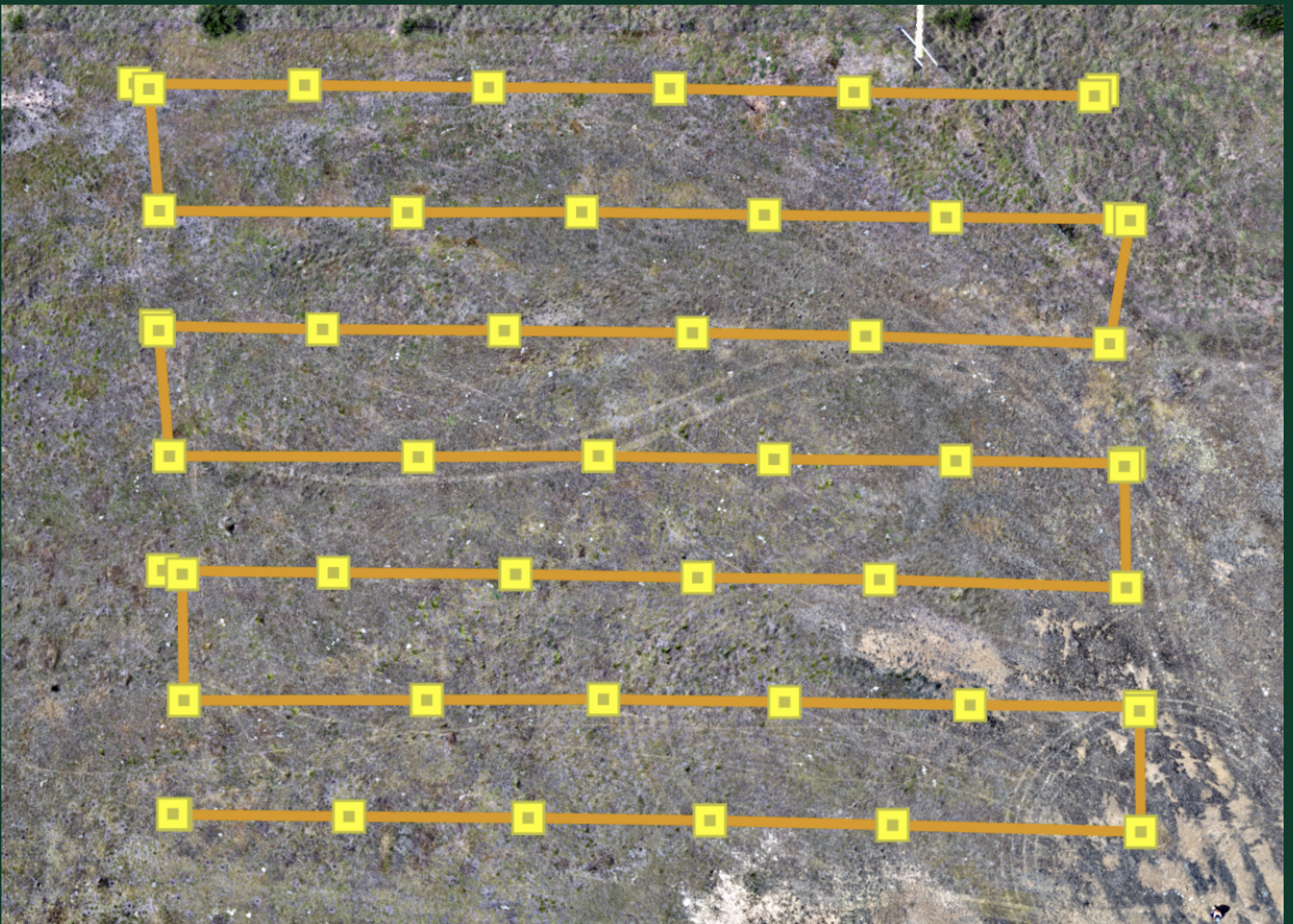
Figure 16. An orthomosaic created using ArcGIS (yellow = image centers; orange = drone flight path)
