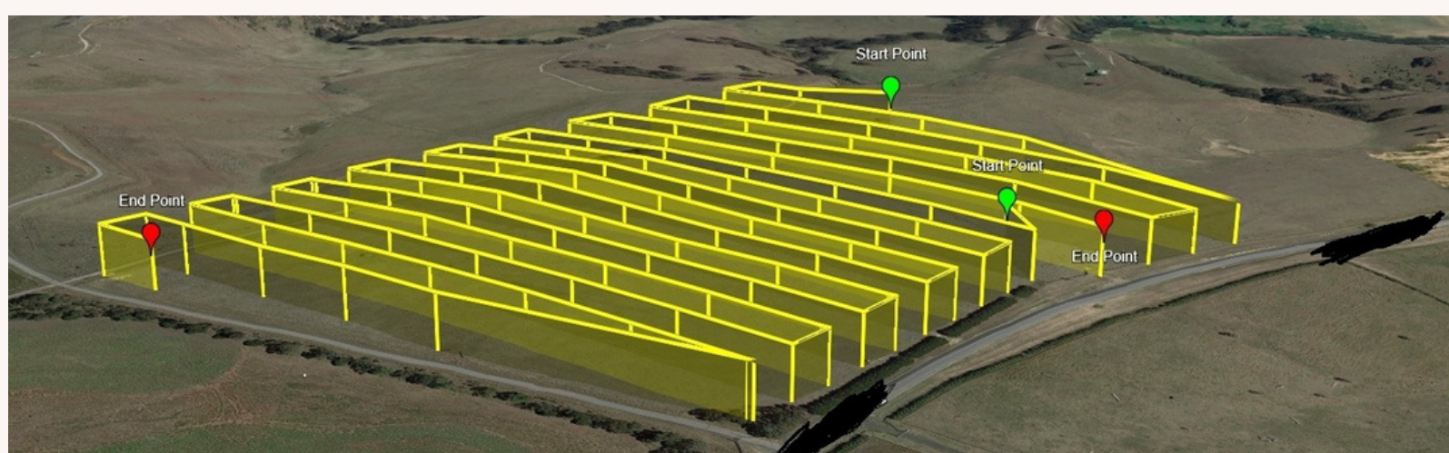
Figure ES-5. Flight path generated by DJI Air 2S software to demonstrates the full flight path
