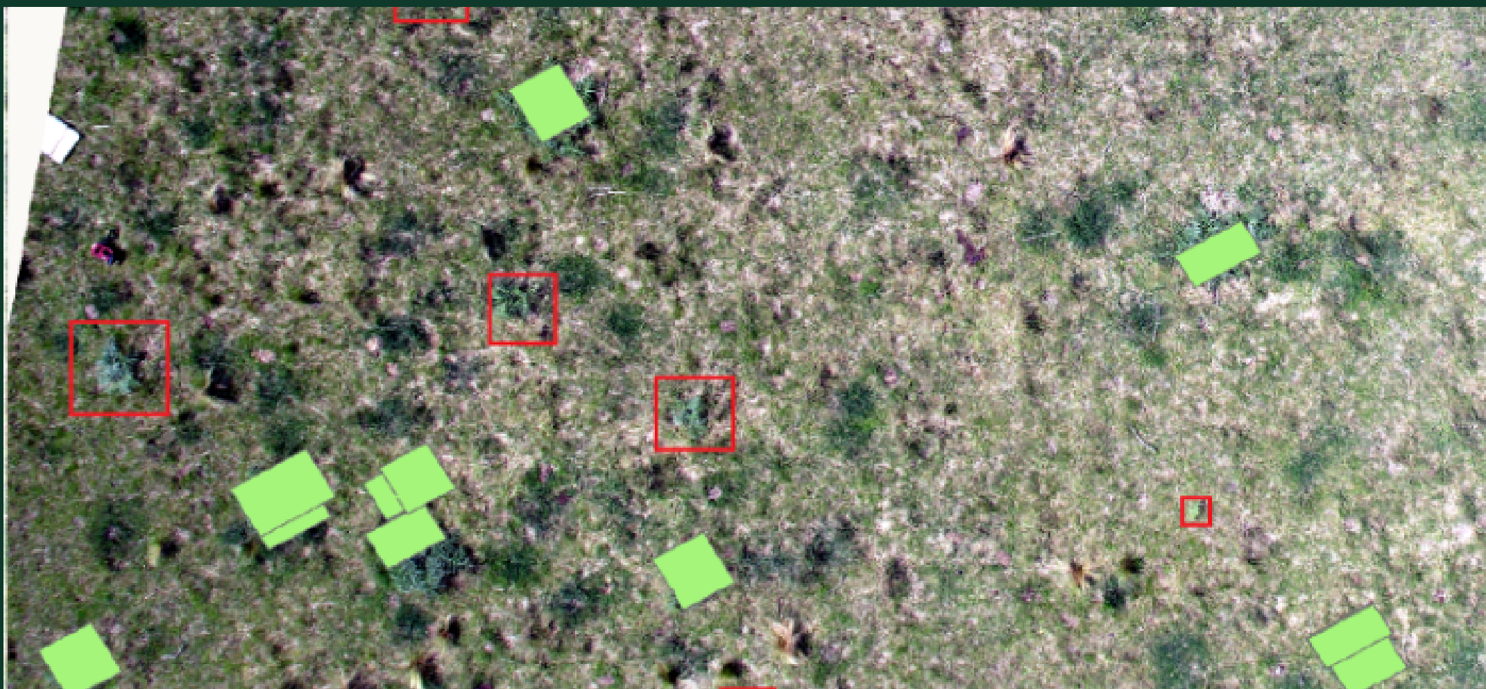
Figure 18. Property 1 with the model's predicted Artichoke Thistle outputs (light green) and missed weeds (red outlines)
