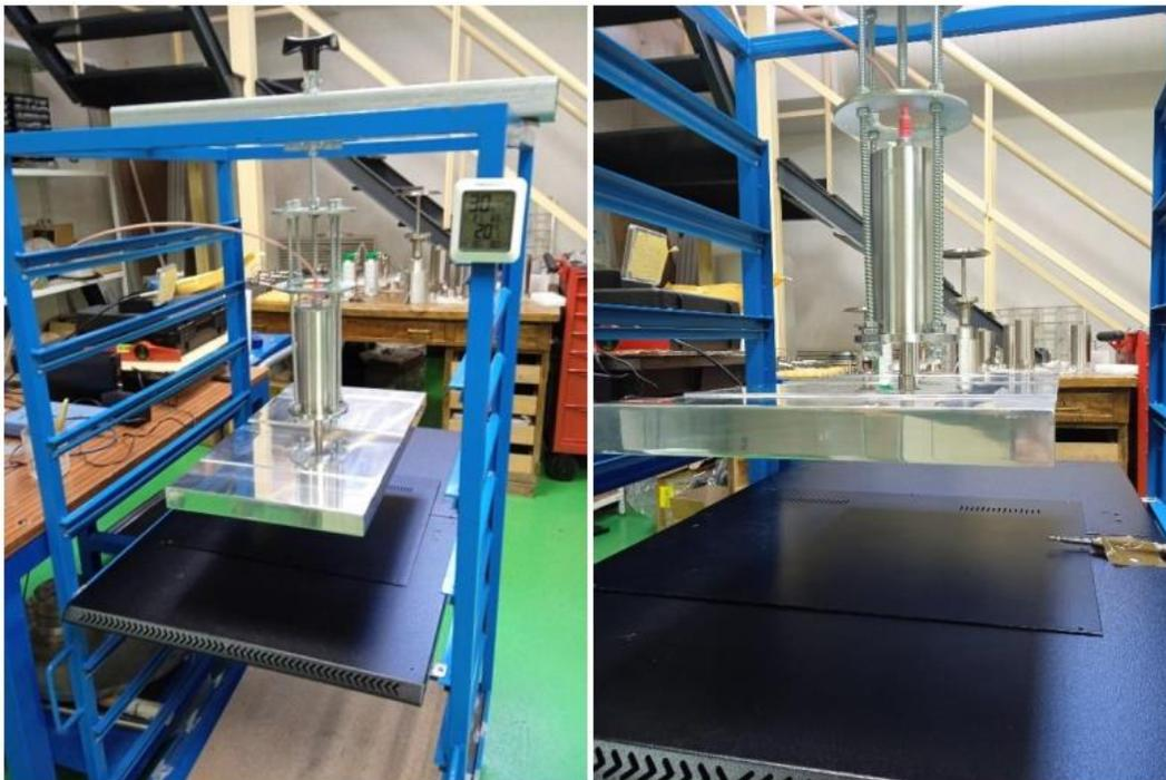
Figure 66. The experimental setup used by Pusonics to measure the acoustic pressure at different distances from the Al plate [120].
