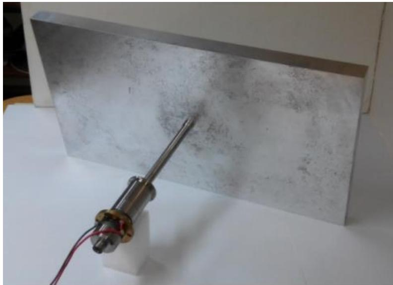
**Figure 63. Airborne power ultrasonic transducer with a rectangular plate radiator [119].**
