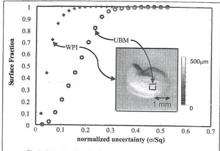
Fig. 5. Plots of surface fraction versus normalized uncertainty, as indicated by the standard deviation at a location normalized by the Sq for all the measurements, for measurements on the alfalfa seed by the WPI-SLM and the UBM. The mean Sq for the WPI-SLM is  $70.1\mu m$  and for the UBM was  $32.7\mu m$ .
