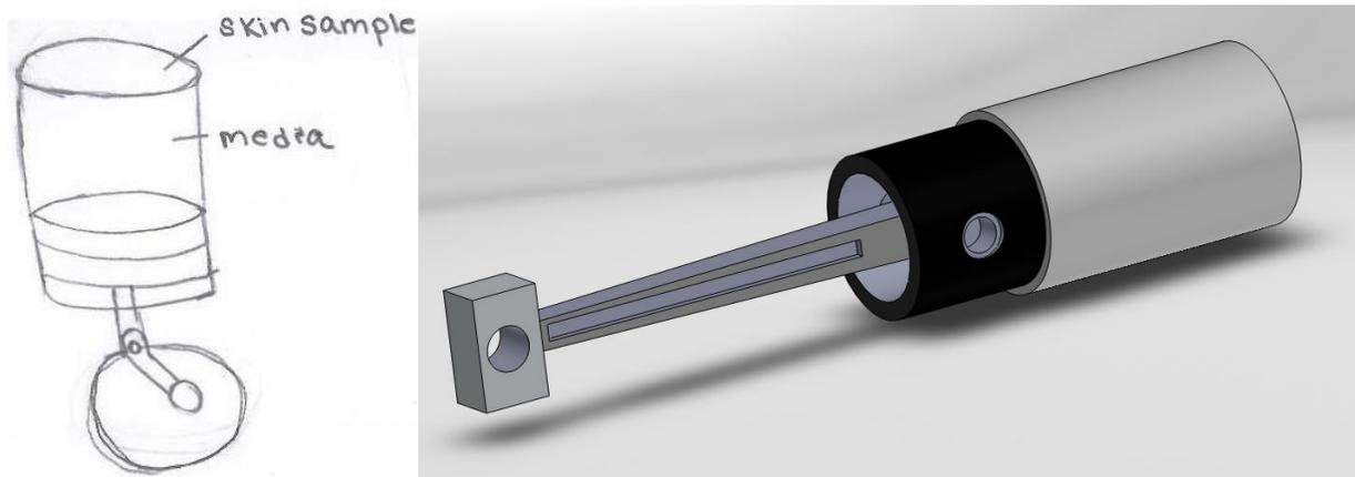
Figure 16: (Left) Initial sketch of The Piston Design, (right) computer-aided drawing
