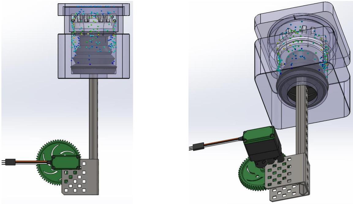
**Figure 33: An illustration of the internal sterile chamber of the bioreactor.**
