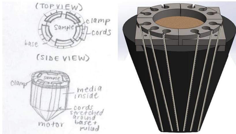
Figure 14: (Left) Expanding Ring initial drawing, (right) computer-aided drawing
