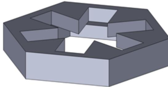
**Figure 22: The cap, a custom part used for fixing the sample.**
