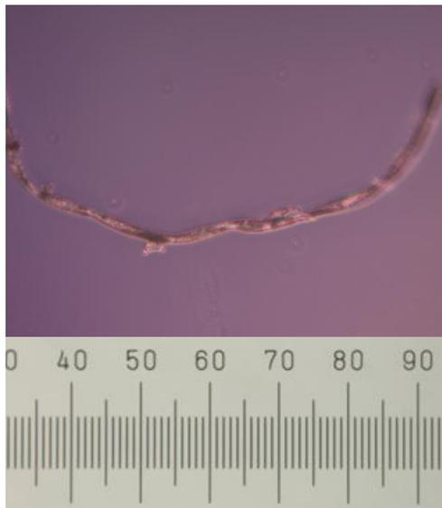
**Figure 34: An example of bacterial contamination at 20x magnification. Compared to a 1mm scale with 100 divisions (0.01 mm).**
