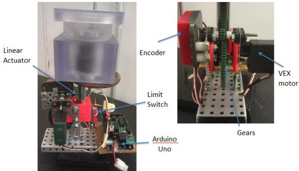
**Figure 23: The rack and pinion setup with motor.**
