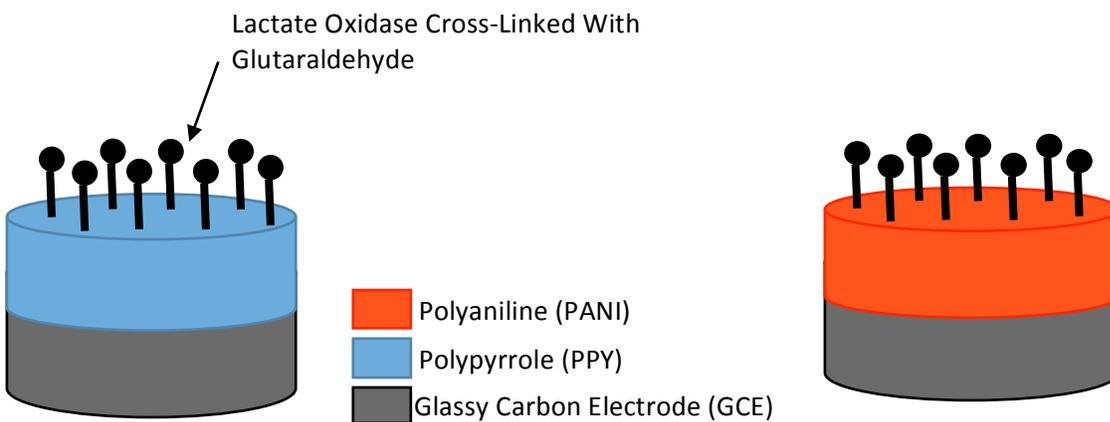
**Figure 5: Single Layer Polymer Deposition**
