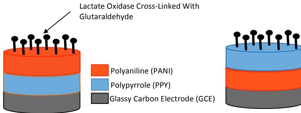
**Figure 6: Dual Layer-by-Layer Polymer Deposition**
