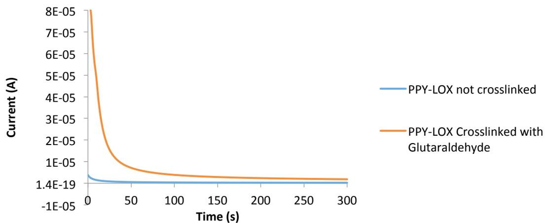
**Figure 12: Amperometry Curves Comparing Addition of Glutaraldehyde**
