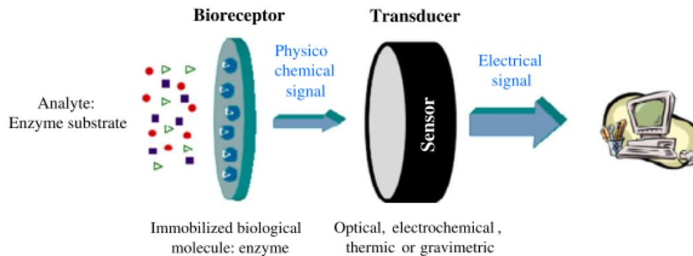
**Figure 2: Scheme of a Biosensor**
