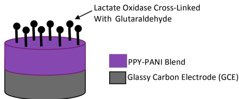
**Figure 7: Co-polymer Blend Deposition**
