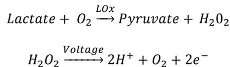
Using lactate oxidase increases the specificity of the biosensor. Other analytes such as glucose and glutamate follow the same breakdown pathway; however lactate oxidase only catalyzes the breakdown of lactate.
