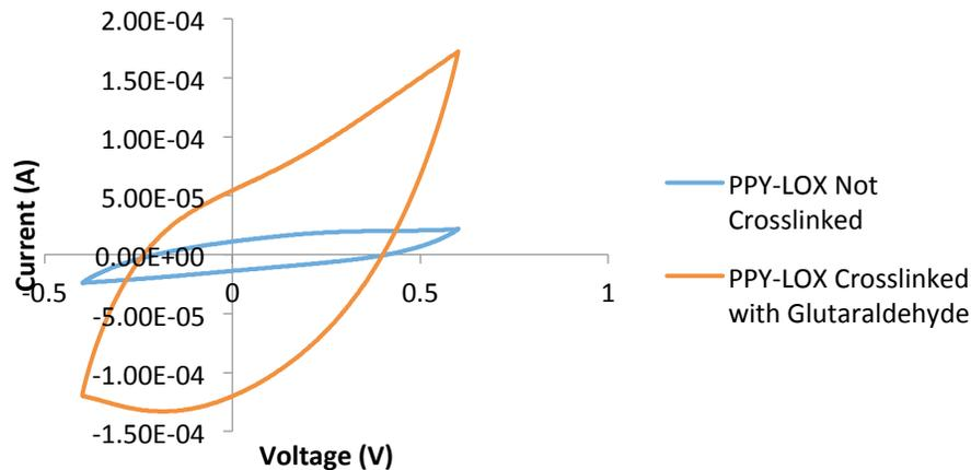
**Figure 13: Cyclic Voltammetry Curves Comparing Addition of Glutaraldehyde**
