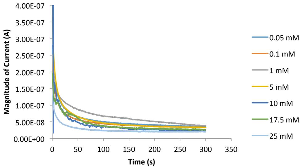
Figure 14: Amperometry Results for PPY-PANI-LOX Crosslinked
