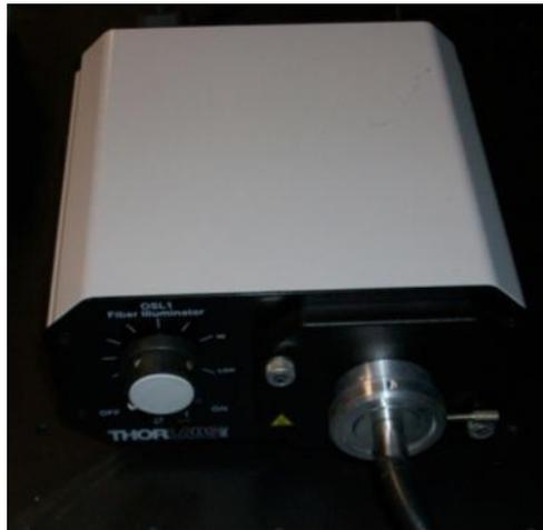
Fig. 44. Thorlabs OSL1 Illuminator with Tungsten Lamp
