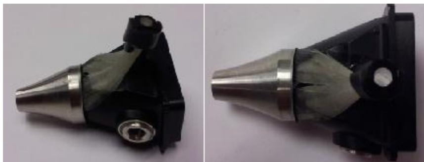
Fig. 20. Exposed Diagnostic Otoscope Fiber Bundle
