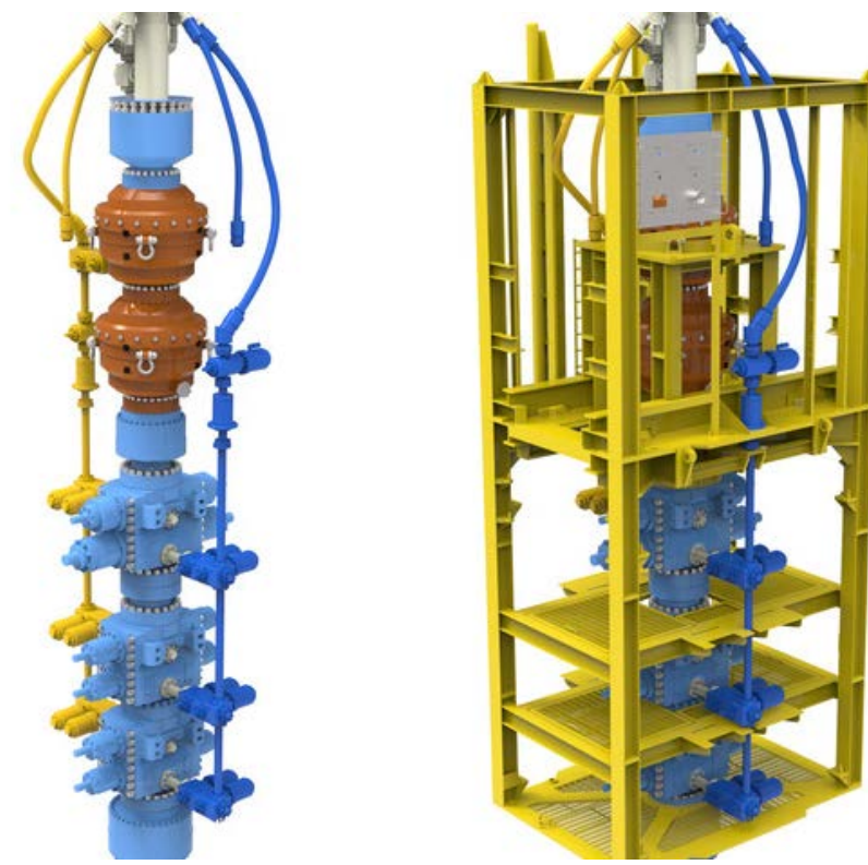
Blow-out preventer with and without frame and control panel
