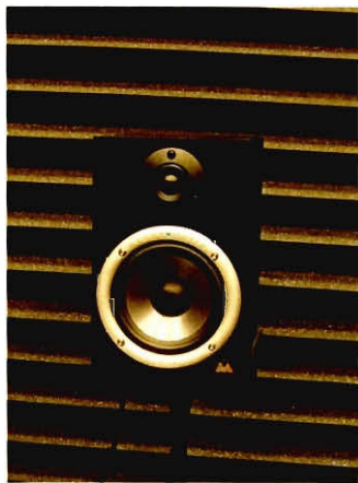
Fig. 3-45 Installed Left Studio Monitor
