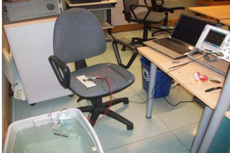
Figure 5.3-1 Test setup in the Lab. It can be seen from the picture that the transmit antenna is position in water and the receive antenna is placed outside of the water. The transmit antenna is used in a parallel combination with different tuning capacitors.
