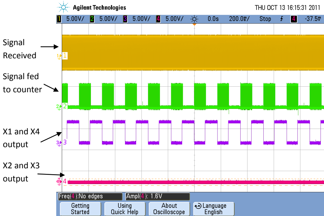
Figure 5.2-12: Oscilloscope image of the input and output of the listening circuit for a 20 kHz signal. The yellow trace is the input square wave, the green shows the input to each counter, and when the counter deactivates, the tag number is displayed at the output of the latch shown by the purple and pink traces, with purple being the least significant bit. For 20 kHz the output is “01” which is used to create fish id number “1001”
