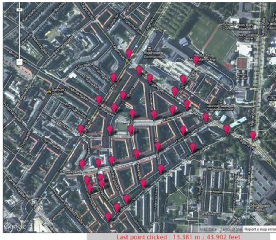
Figure 22. Mapping of the waypoints used to construct a contour map of the terrain (Daft Logic, 2011).
