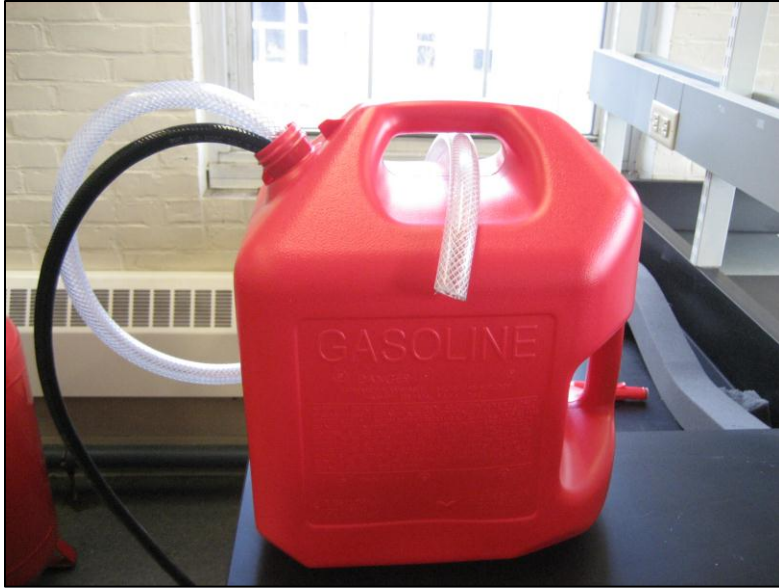
Figure A5. Compressed air apparatus to remove residual fuel vapors.
