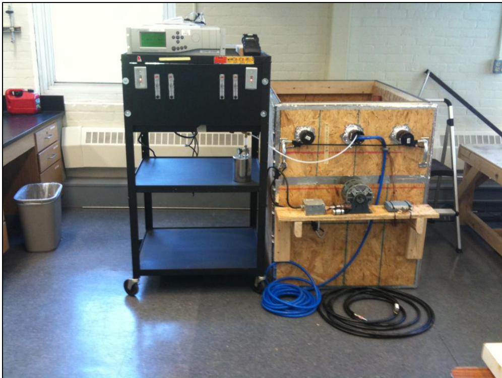
Figure A6. Environmental chamber with vapor testing instrumentation.
