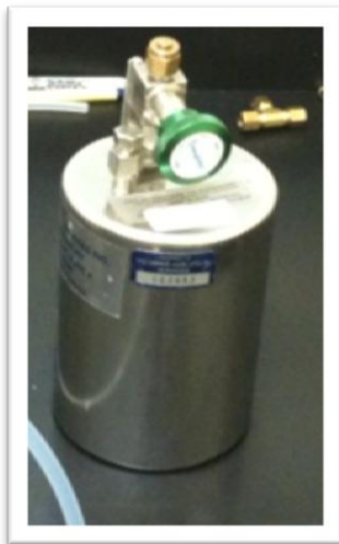
Figure A10. Summa canister used for grab sample acquisition and laboratory analysis.
