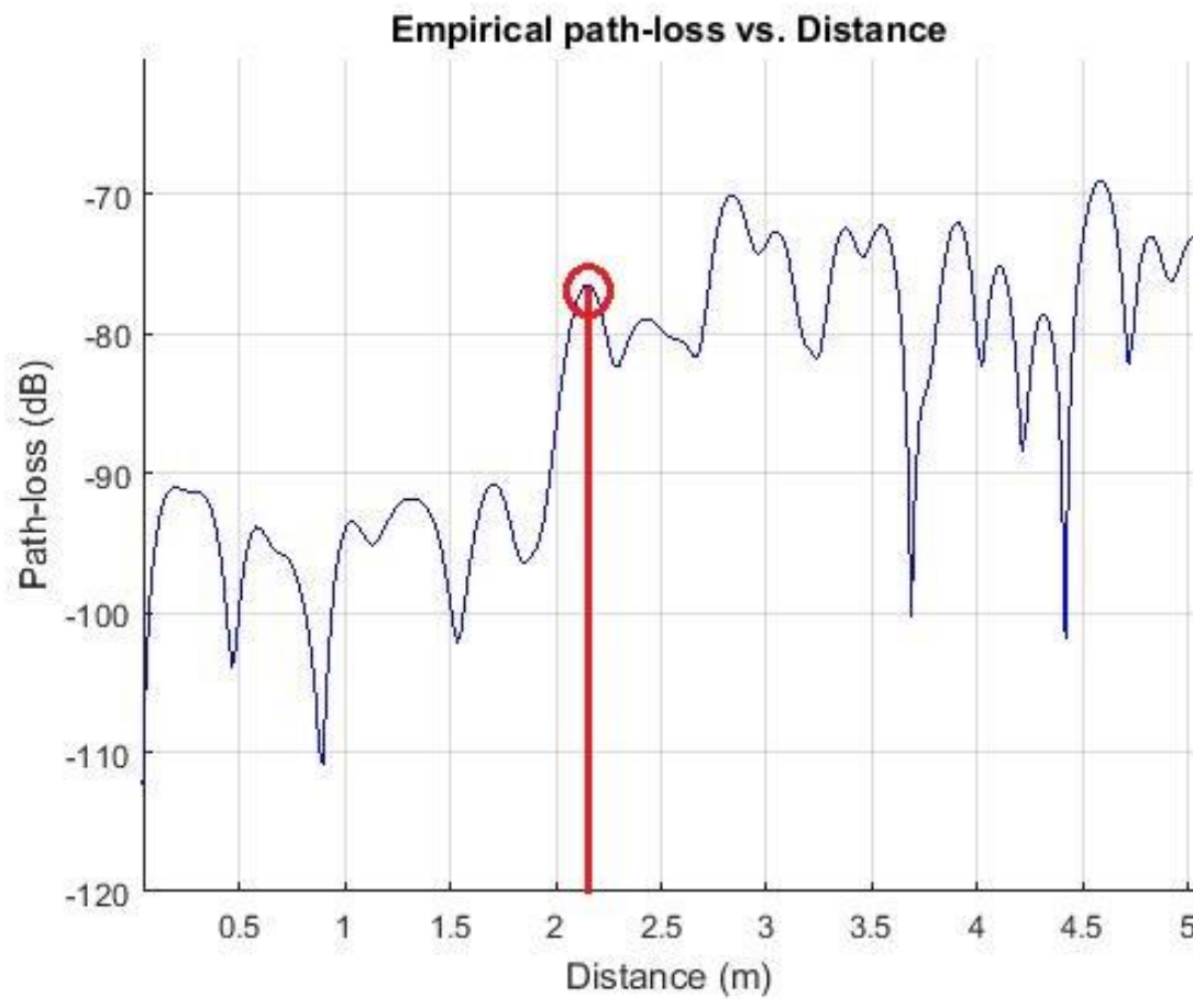
Figure 4.8 Measurement campaign – Blocking diffraction path on one side of the metallic door using an absorber.
