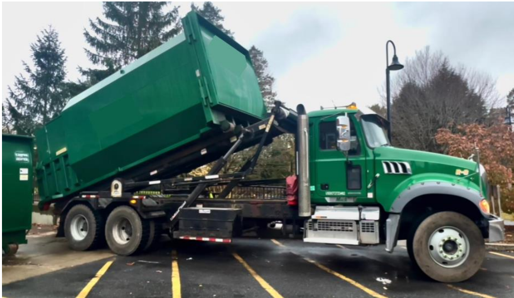
Figure 6: Garbage truck picking up the compactor at the Rubin Campus Center at WPI
