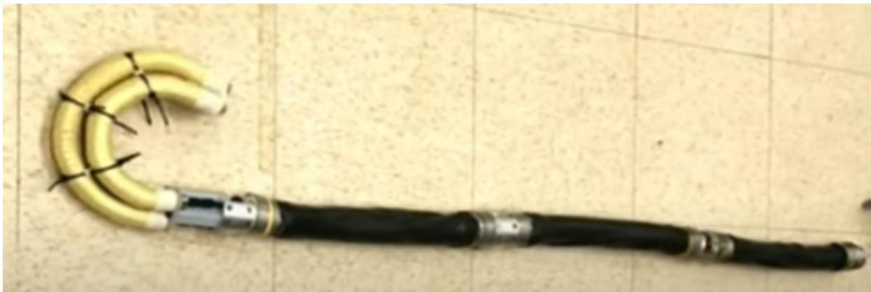
***Figure 10: GE Pipe-worm (Programmable Worm for Irregular Pipeline Exploration) Robot [18]***
