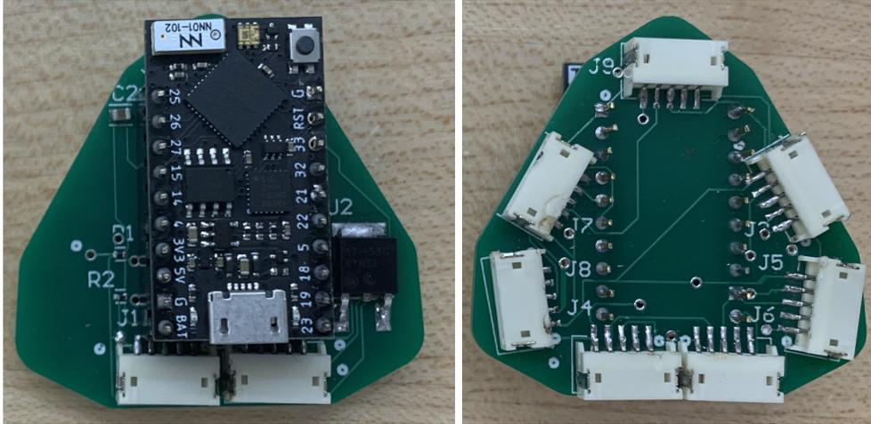
**Figure 63: First Iteration Mainboard PCB**
