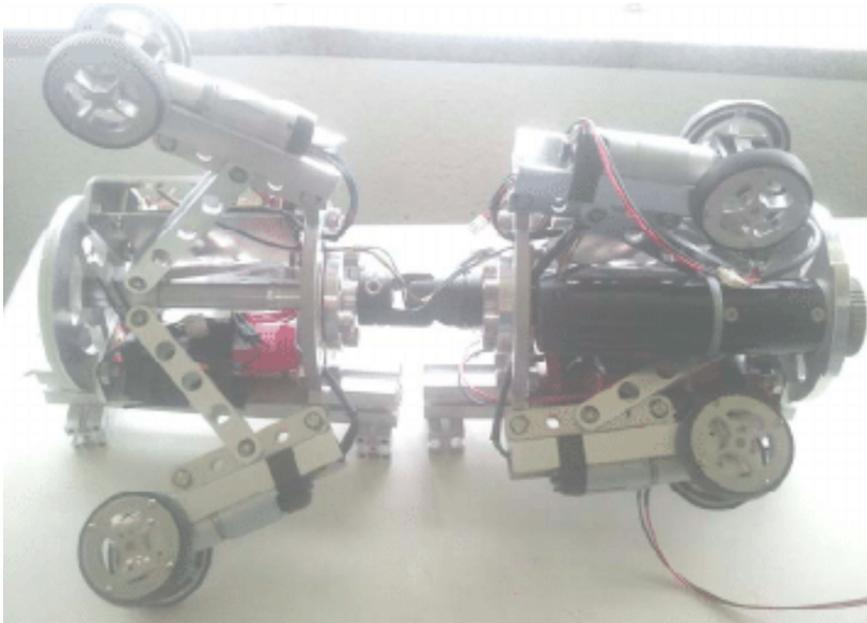
***Figure 9: Pukyong National University Wheeled Pipe Inspection Robot [17]***
