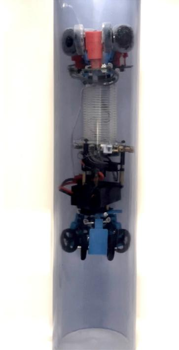
*Figure 91: Vertical Pipe Traversal*
