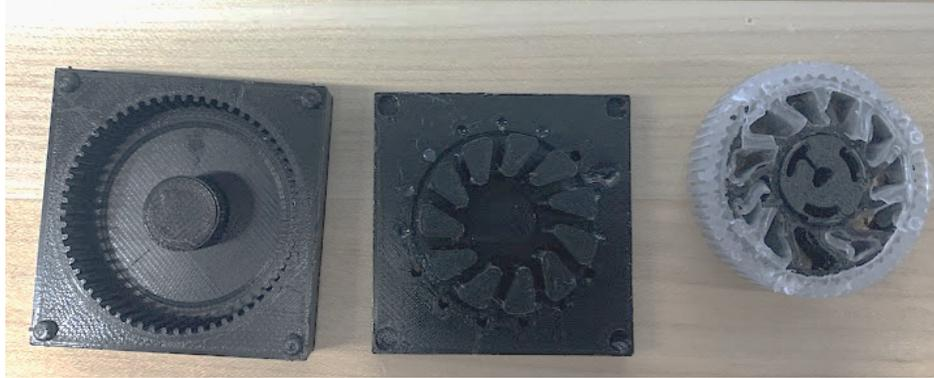
*Figure 42: Compliant Wheel v2 Mold Result*
