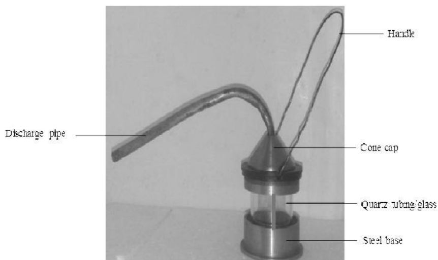
Figure 3: Lantern Retort (Amankwah and Ofori-Sarpong, 2010)
