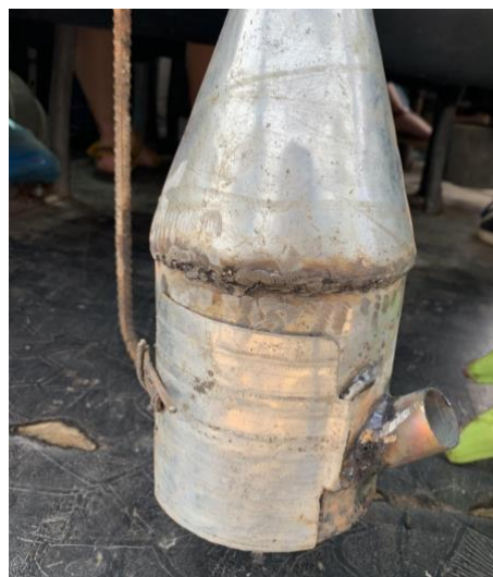
Figure 16: Modified Burning Vessel
