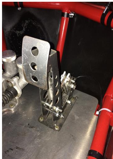
Figure 65: Modified Foot Control
