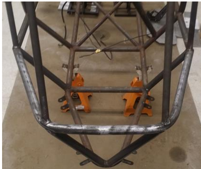
Figure 30: Actual Frame after Hubb Equipment Welding
