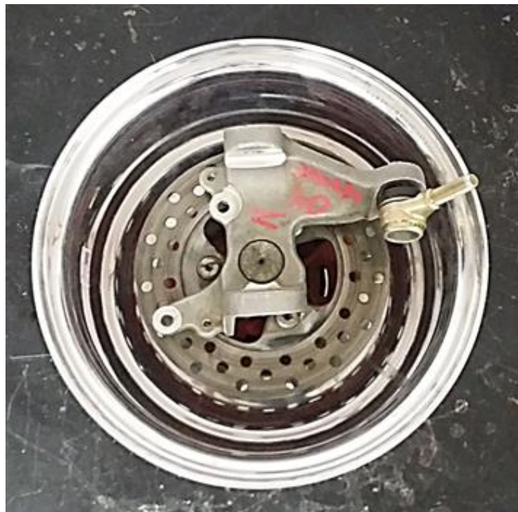
Figure 21: 2004 KFX-400 Hub Assembly Mounted to Rim
