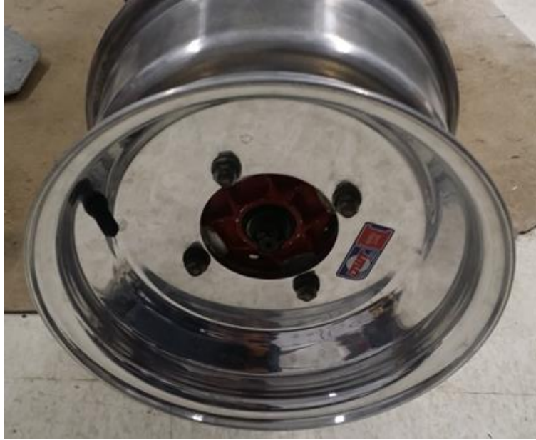
Figure 20: 2004 KFX-400 Hub Assembly Mounted to Rim
