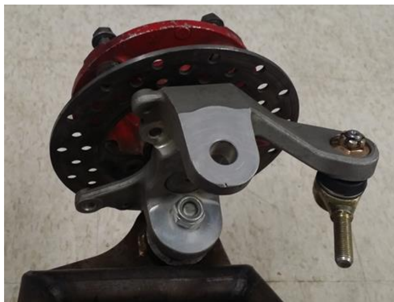
Figure 19: 2004 KFX-400 Hub Assembly
