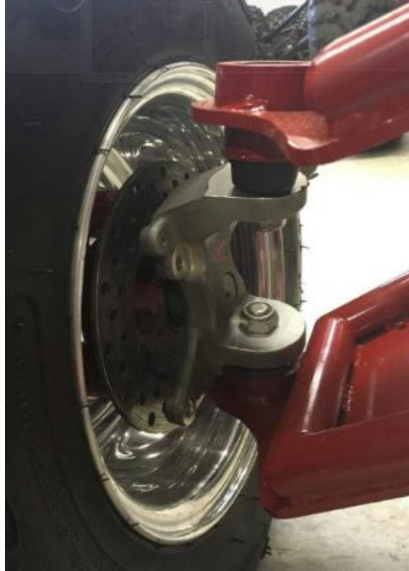
Figure 25: Complete Tire, Wheel Spacer, and Hub Assembly
