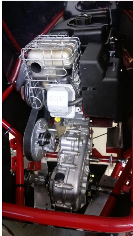
Figure 62: Final Orientation of Drivetrain
