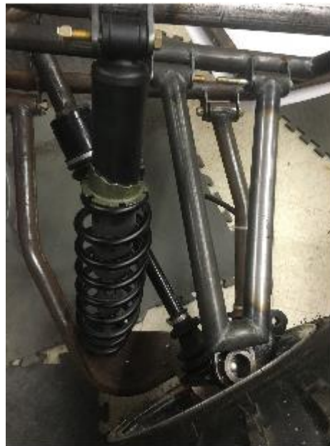
Figure 34: Finalized Rear Suspension
