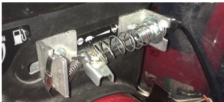
Figure 66: Throttle Cable Mounting System
