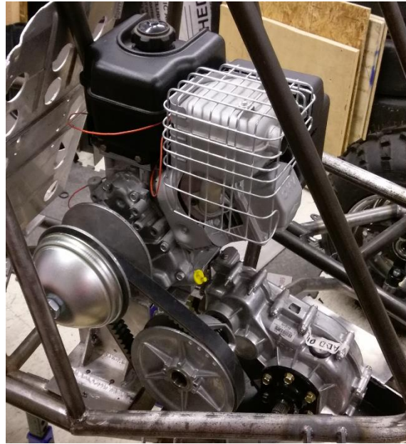
Figure 43: CVT Mounted to the Model 20 Engine
