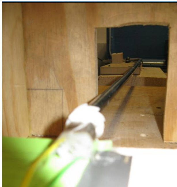
FIGURE 24 - INTAKE PIPE INTO TURBINE HOUSE
