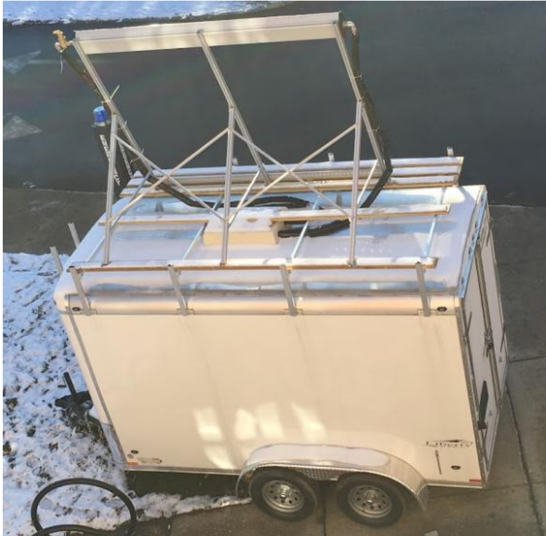
Figure 29: Running the Steel Tubing into the Trailer
