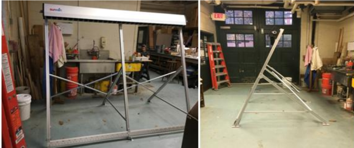
Figure 26: Assembled Solar Collector Frame
