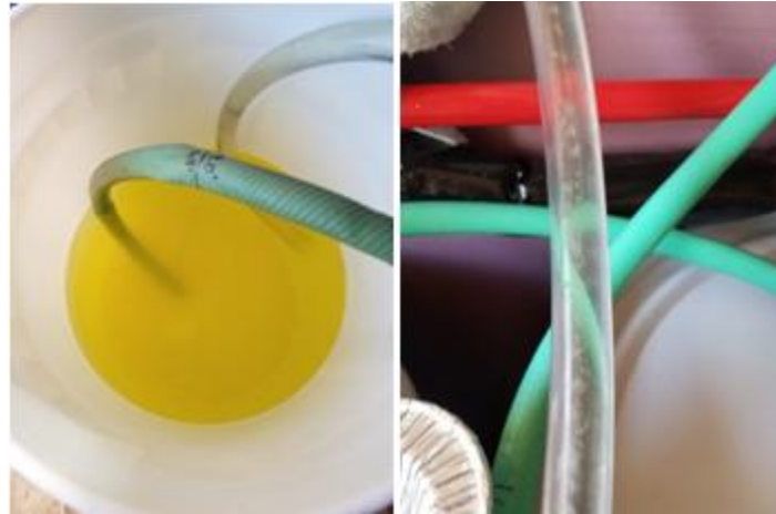
Figure 37: Glycol Bucket (Left) and Bubbles in the Clear Hose (Right)
