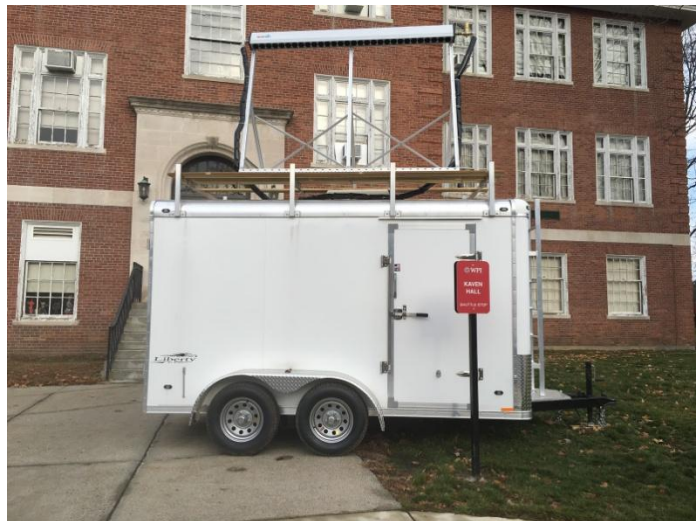
Figure 27: Solar Collector Frame Mounted to the Trailer
