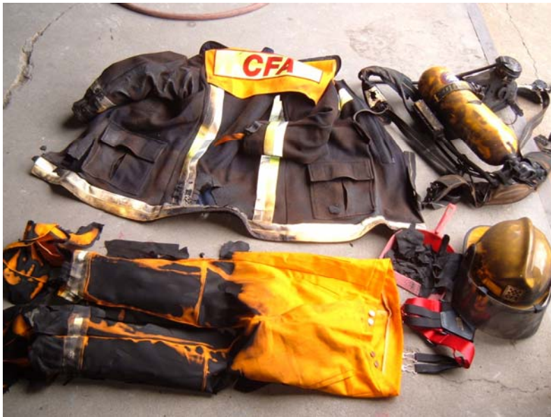
Figure 4-35: Australian Ensemble 2 Post-Test
