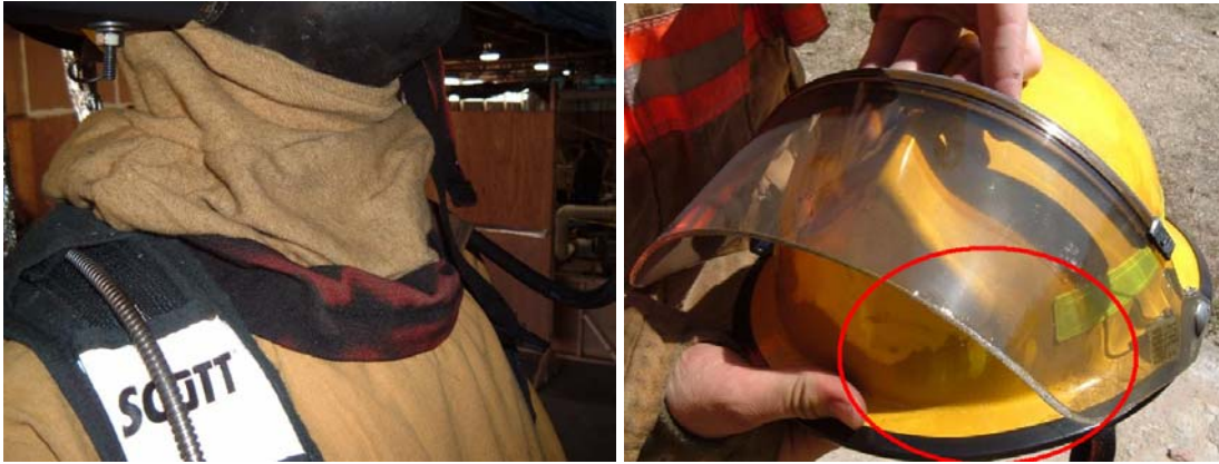
Figure 0-15: Navy Ensemble Neck Discoloration and Helmet Deformity after Initial Doorway Test
