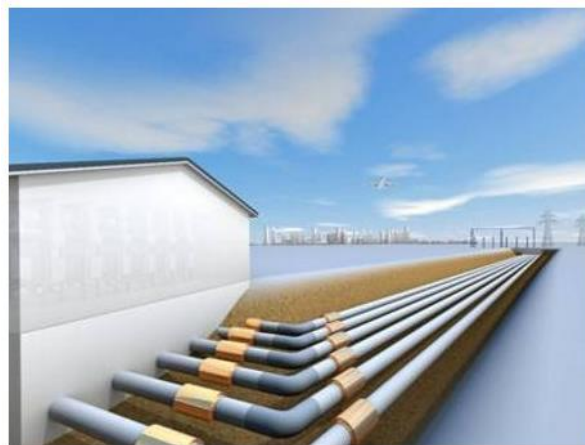
Figure 20: Image of the Gas Insulated Lines (Alpiq, 2014).
