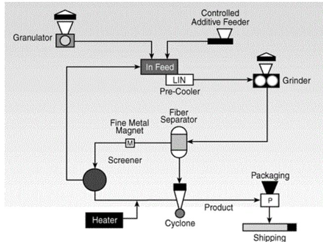
Figure 10 - Cryogenic Grinding Process (Tire Recycling Made Simple, 2012).
