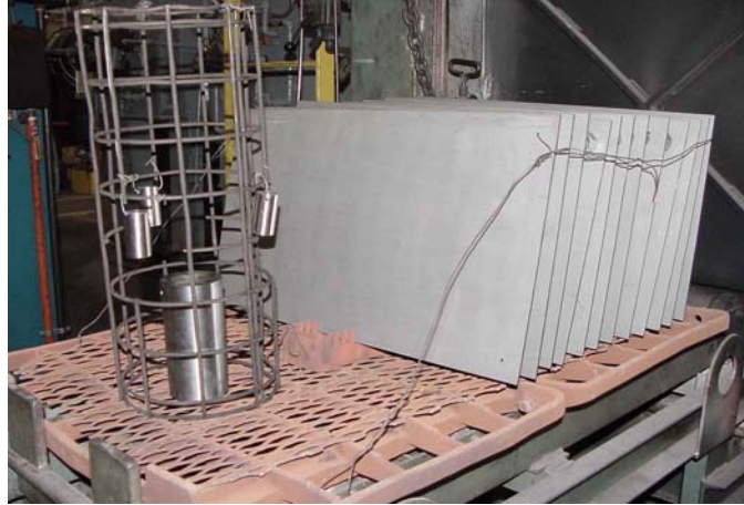
Figure 3. Experimental setup: test coupons, carbon step bar and additional surface area.
