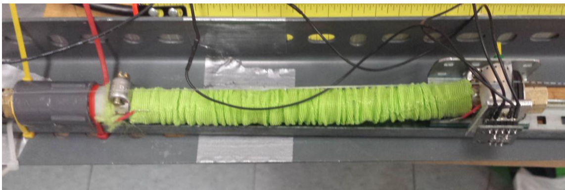
Figure 4: Hydro Muscle during control tests.
