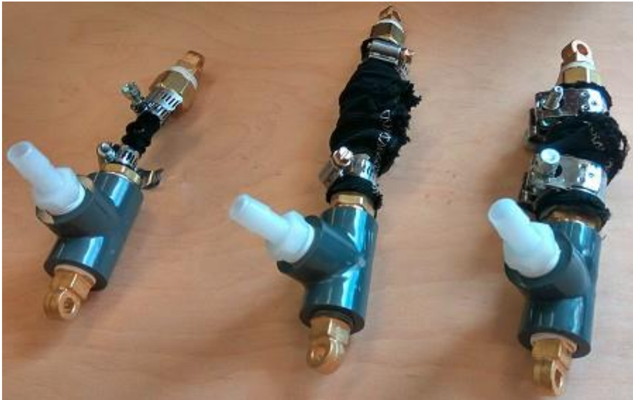
Figure 26: Hydro Muscle based muscle fibers; from left to right the fibers are the Tibialis Anterior, the Gastrocnemius, and the Soleus
