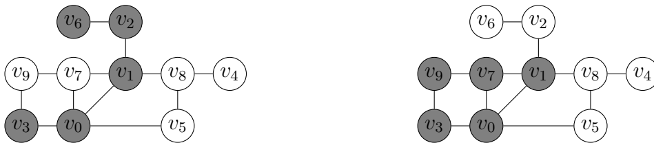
Figure 2.5: Left: A graph with a path from v_3 to v_6 . Right: A graph with a cycle formed by the sequence of edges \{(v_0, v_3), (v_3, v_9), (v_7, v_9), (v_1, v_7), (v_0, v_1)\} .
