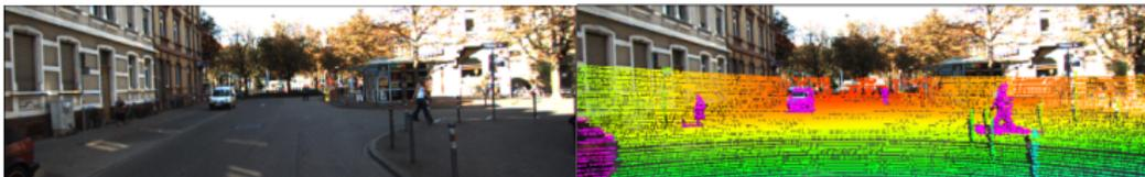
a. Camera Image, b. LIDAR front projection on image with labels
