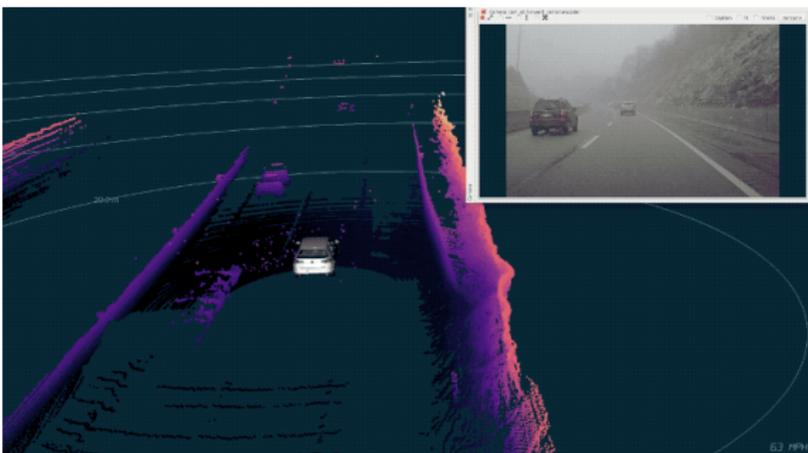
Lidar is sensitive enough to detect snow, making it more difficult to identify important objects.
