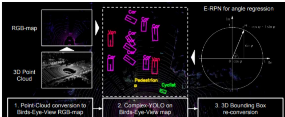
Complex-YOLO [SMAG18] uses bird's eye view projection for detection
