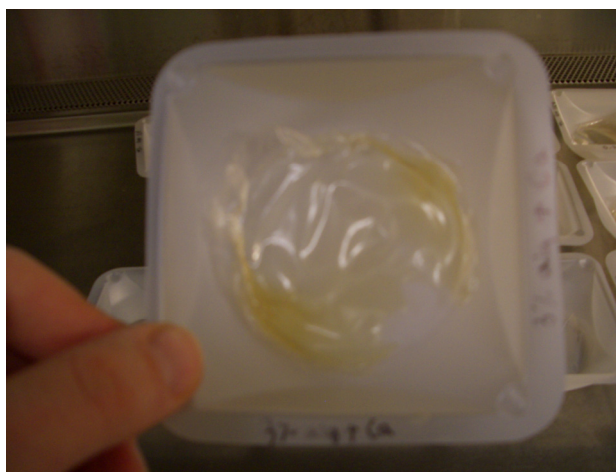
Figure 19: Dry 3% Alginate + Calcium Nitrate – brittle and curled gel, non-homogeneous
