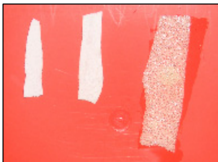
Control Encap.Terpene Free Terpene Figure 39: Terpene Resistance Test – Polyurethane Foam sample
