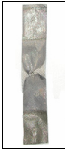
Figure 33: Acticoat™ 7 specimen after testing.
