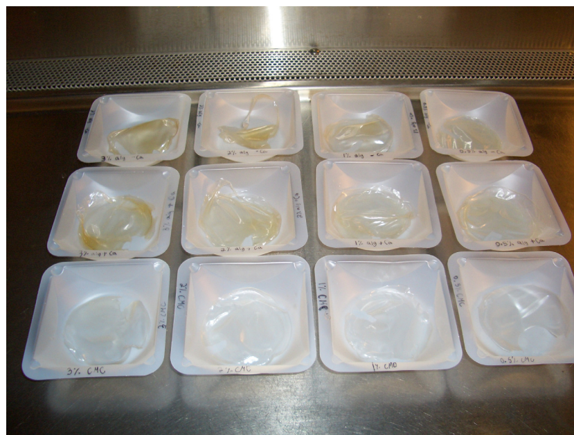
Figure 18: Dry Alginate and CMC hydrocolloids, (top row –alginate control, middle row – alginate + terpene, bottom row – CMC control, left to right are 3%, 2%, 1%, 0.5% formulations by row)
