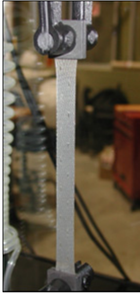
Figure 32: SilvaSorb™ specimen during tensile test
