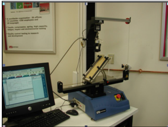
Figure 27: Complete test configuration for 135 degree peel test
