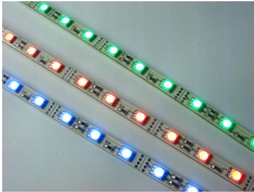
Figure 81 – Red, Green, & Blue LED Light Strips
