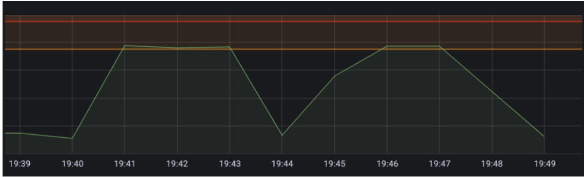
Figure 37: Grafana graph showing the CPU usage on the newer 128-core machine when running TLS-Perf with TLS version 1.2 (on the left) and then running TLS-Perf with TLS version 1.3 (on the right)
