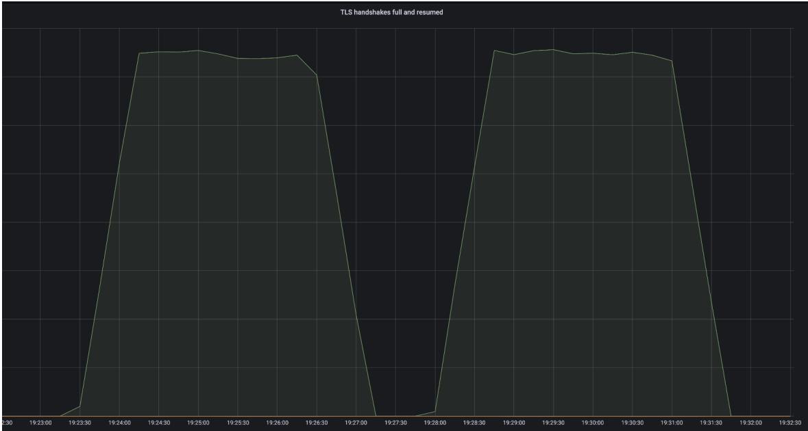
Figure 36: Result from running against the 72-core machine. Grafana graph showing the number of TLS handshakes accepted when running TLS-Perf with TLS version 1.2 (on the left) and then running TLS-Perf with TLS version 1.3 (on the right)
