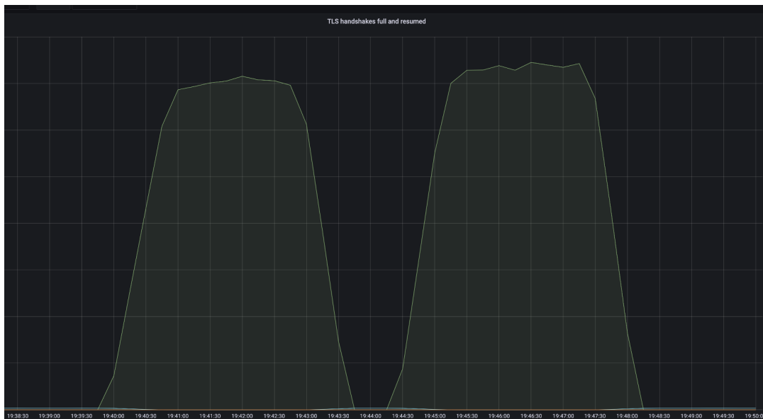
Figure 38: Result from running against the newer 128-core machine. Grafana graph showing the number of TLS handshakes accepted when running TLS-Perf with TLS version 1.2 (on the left) and then running TLS-Perf with TLS version 1.3 (on the right)
