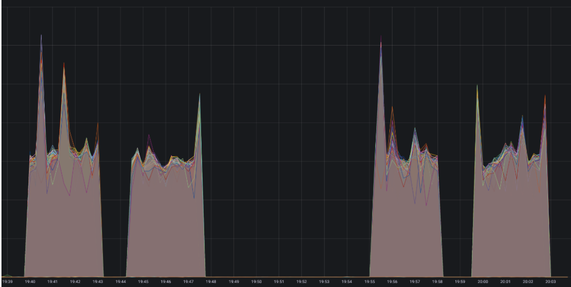
Figure 41: Grafana graph showing the latency of the h2o event loop when running the TLS-Perf test against the 128-core machine varying number of generators (four on the left, five on the right) and TLS version (first and third bump being TLS 1.2, and second and fourth being TLS 1.3)
