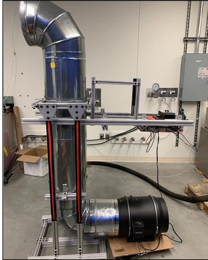
Figure 12: Fully assembled firebrand generator
