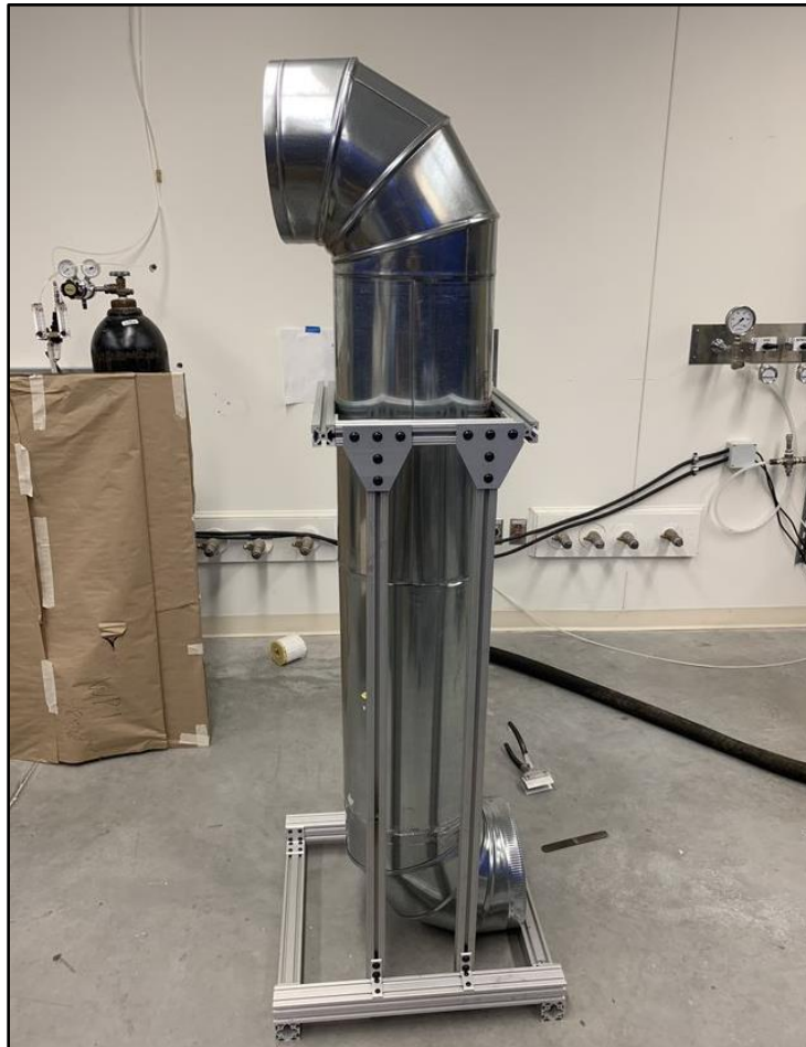
Figure 9: Initial construction of the main body of the firebrand generator
