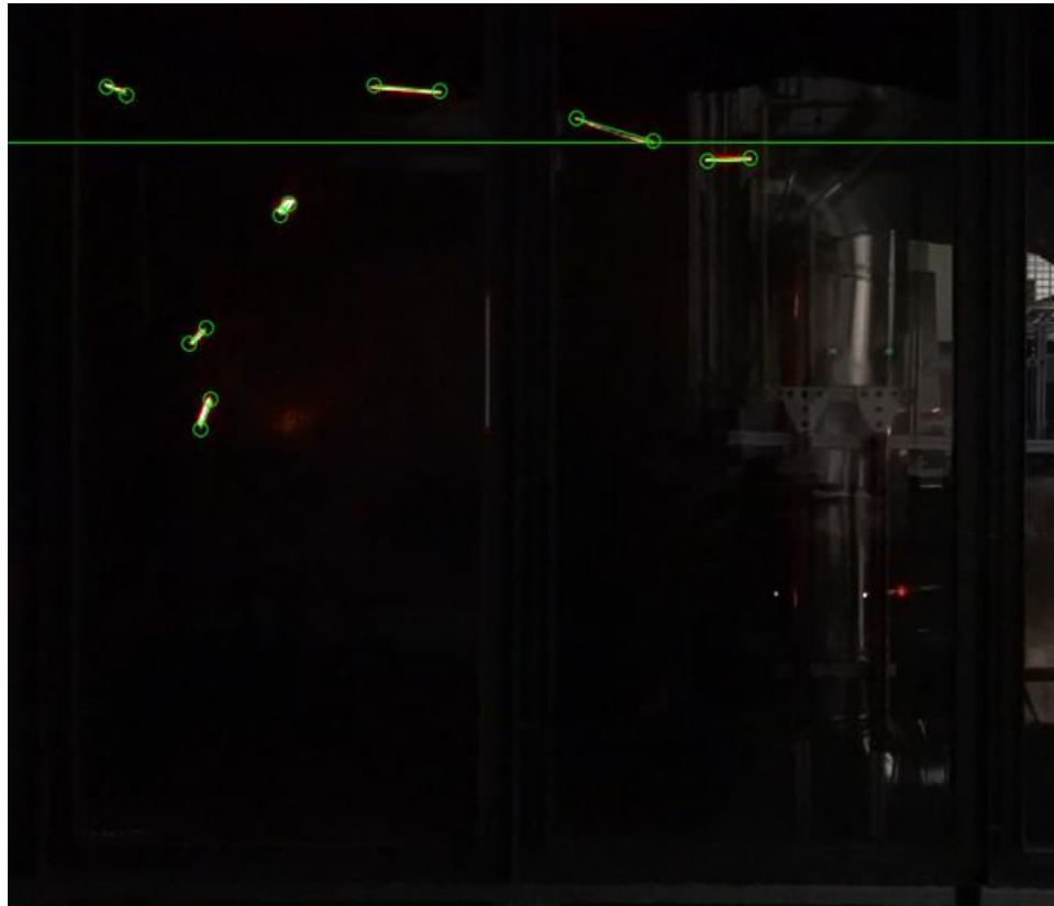
Figure 19: Example of firebrand streaks being measured using MATLAB
