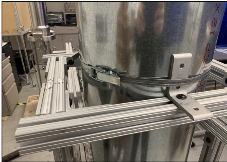
Figure 13: Upper support and duct mount
