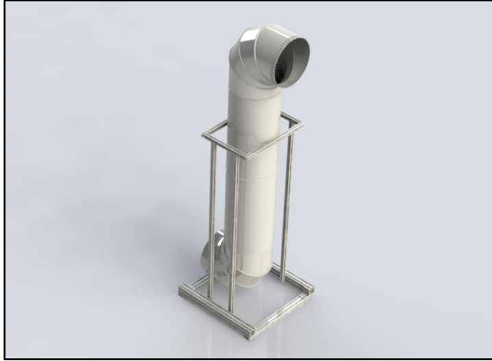
Figure 8: SolidWorks render of the main body of the firebrand generator
