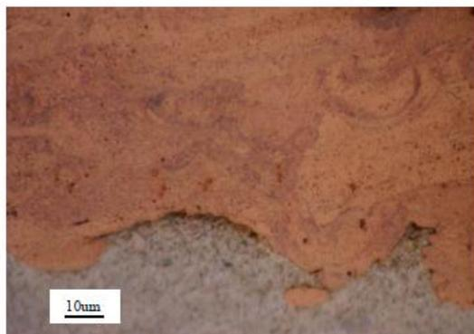
Figure 4 : Cross sectional view of the cold sprayed copper nano powder deposit.
