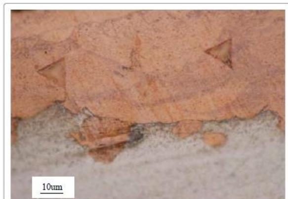
Figure 7: Nano hardness indents on the cross sectional of a cold sprayed nano powder deposit.
