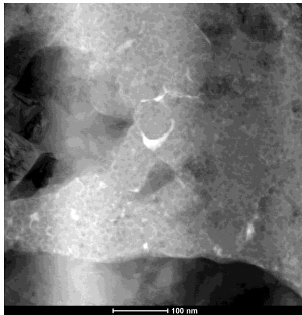
Figure 5: STEM image of the nano copper coating showing the nanostructured particles
