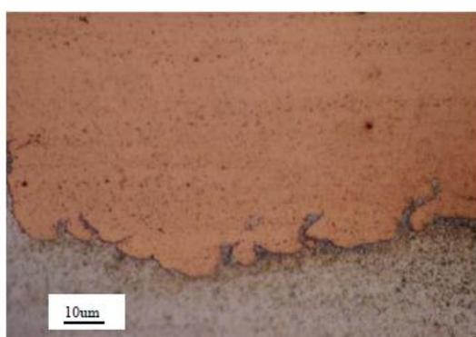
Figure 5 : Cross sectional view of the cold sprayed copper conventional powder deposit.
