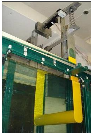
Figure 8: Vortex Induced Vibration for Aquatic Clean Energy (VIVACE) [7]
