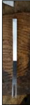
Figure 22: Top View of Link CD to Highlight the Slot at the Bottom of the Piece
