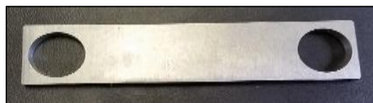
Figure 20: Finished Link BC Component
