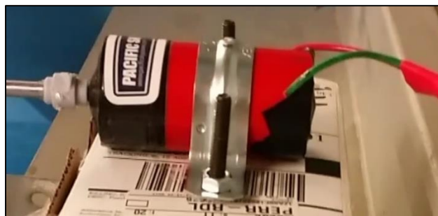
Figure 44: Pacific Sky Power Wind Turbine Generator Connected to the Crankshaft
