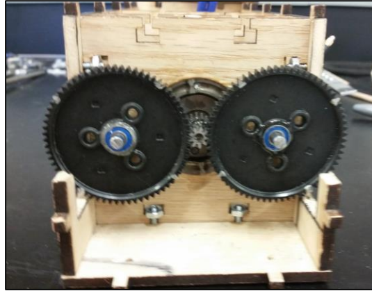
Figure 11: Dual Crank Gear Arrangement with Fixed Motor Gear (9:1 Gear Ratio)
