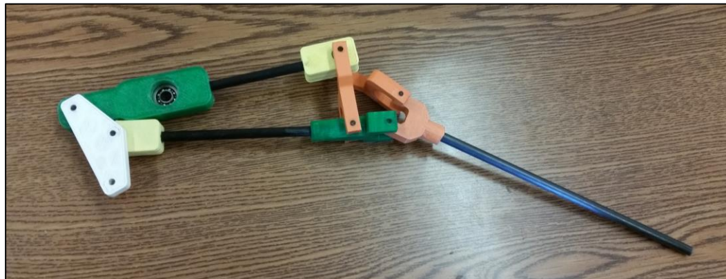
Figure 2: 3D Printed Linkage with Jointed Motion
