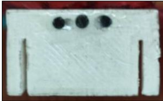
Figure 18: CAD Designed and 3D Printed Connector for Tail
