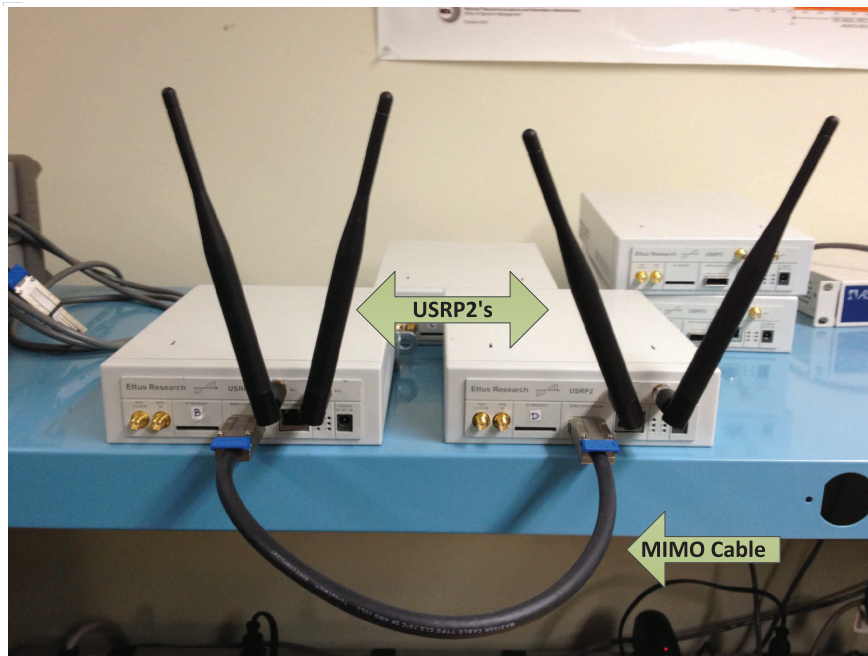
Figure 3.5: USRP2 MIMO cable connecting two USRP2 devices. This cable is used to couple local oscillators together to phase align output samples.
