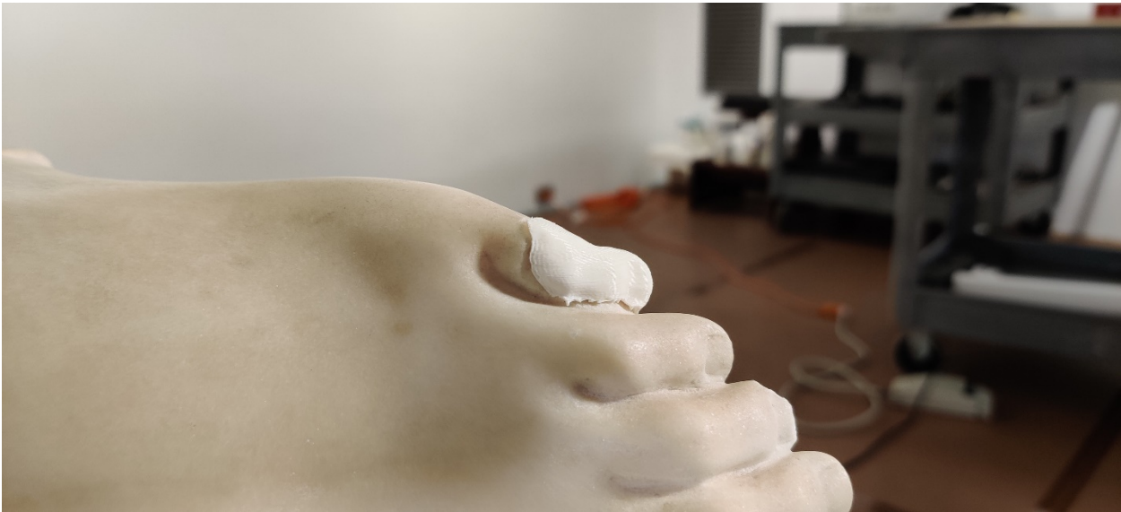
Figure 5.9: Poor fit around the break site caused by the low-quality print settings. Top View.
