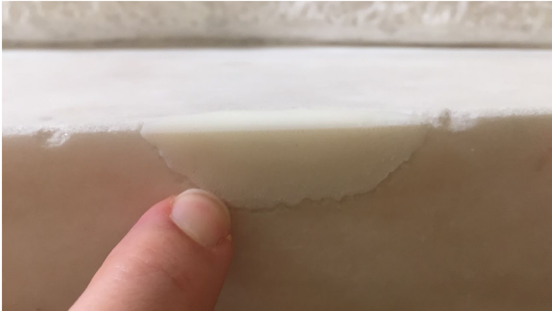
Figure 4.26: Printed pedestal piece fitting into the missing chunk of the statue. Front View.
