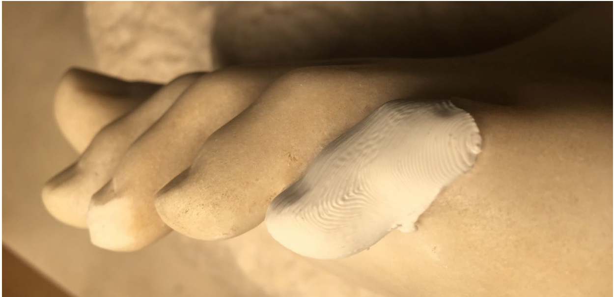
Figure 5.8: Second printed iteration of the right pinky toe. Despite the low print quality, the pinky toe looks aesthetically correct with the rest of the foot.
