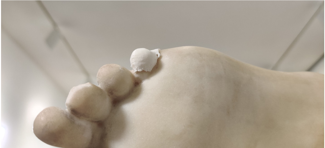
Figure 5.10: Poor fit around the break site caused by low-quality print settings. Bottom view.
