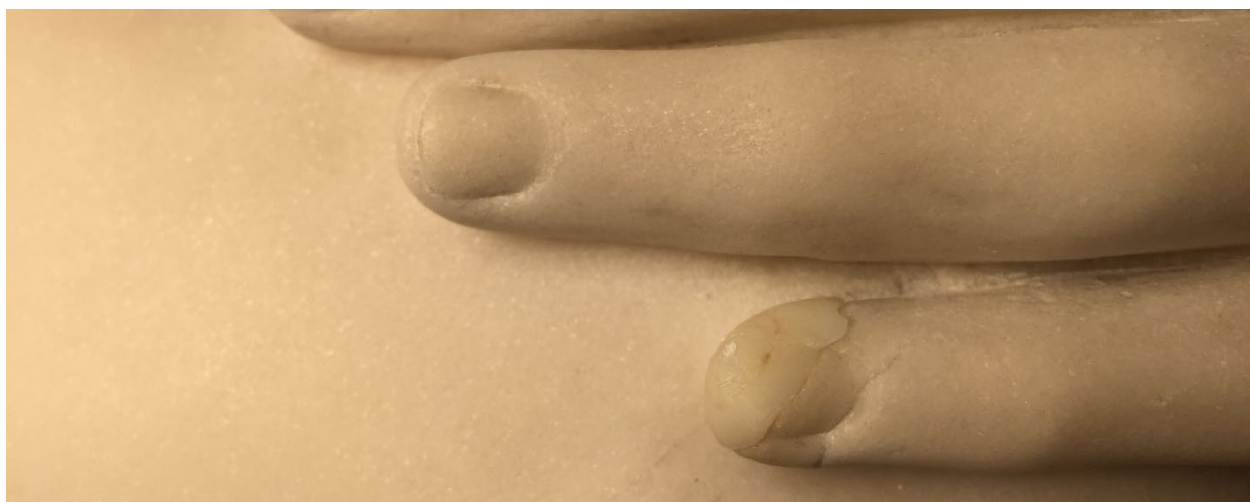
Figure 5.14: The last printed iteration of the fingertip nicely integrating with the rest of the hand, a small seam is visible.
