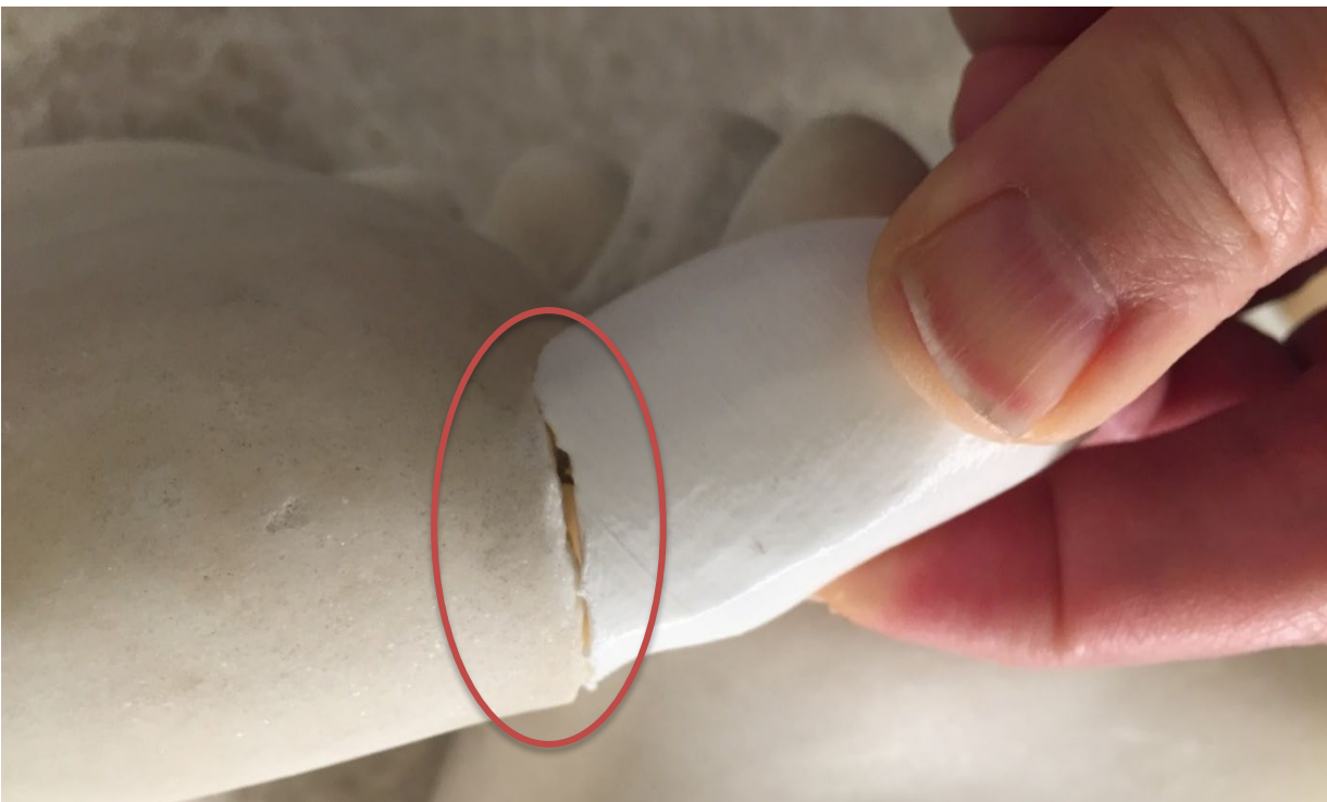
Figure 5.3: An early iteration of the right big toe, with fit issues around the break surface marked in a red circle.
