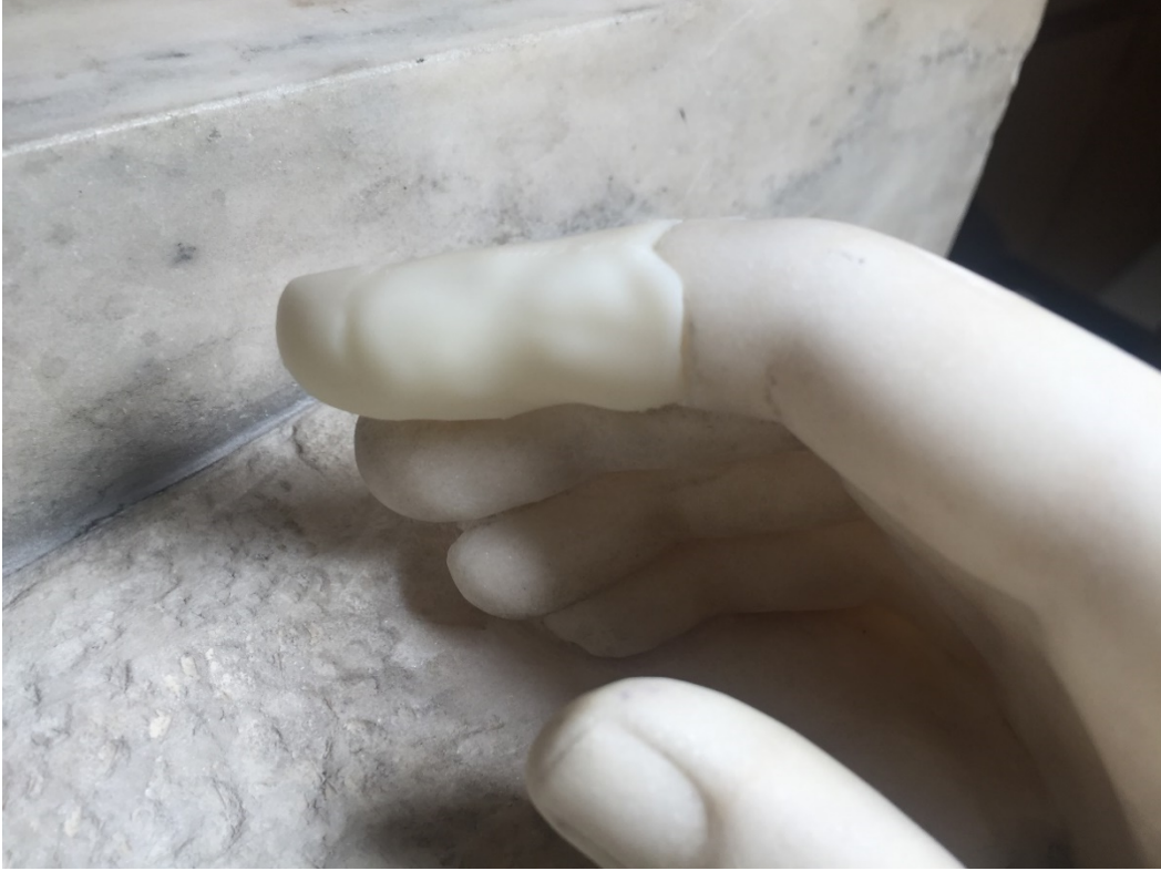
Figure 4.28: Improved Finger compared to the previous iteration. Back view.
