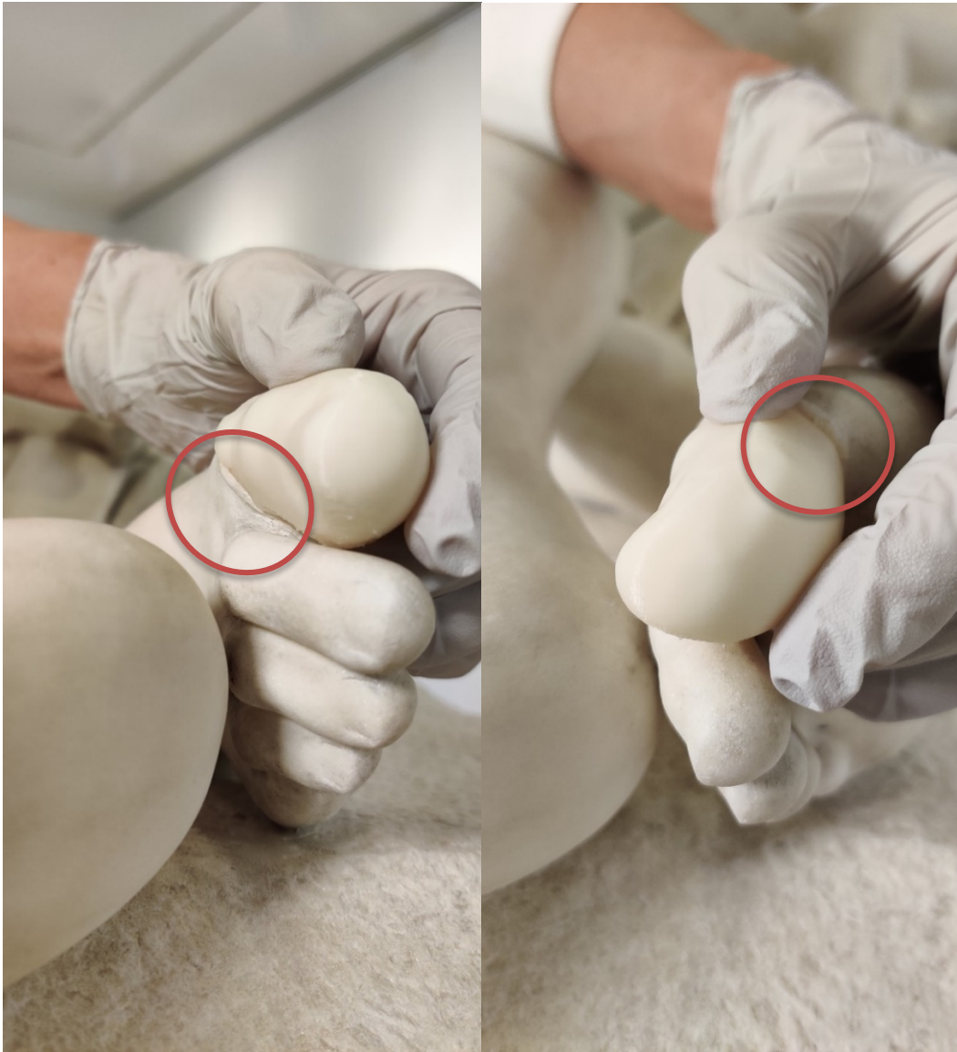
Figure 5.1: The final printed iteration of the toe, with circles marking the fit issues around the broken surface.
