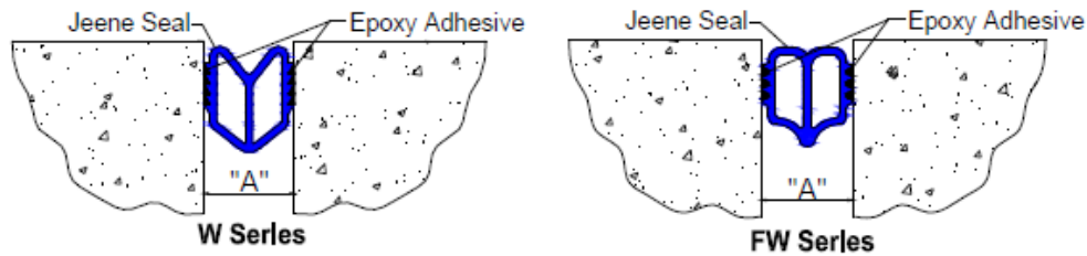
Figure 5: Jeene-Bridge Sealing System (WBA Corp, 2007)
