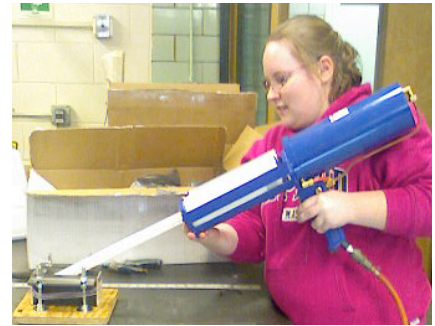
Figure 10: Sealant Pouring Method
