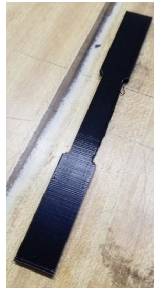
Figure 3.8. Group two specimen printing configuration (large side up).
