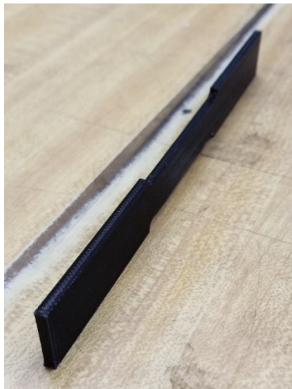
Figure 3.7. Group one specimen printing configuration (thin side up).
