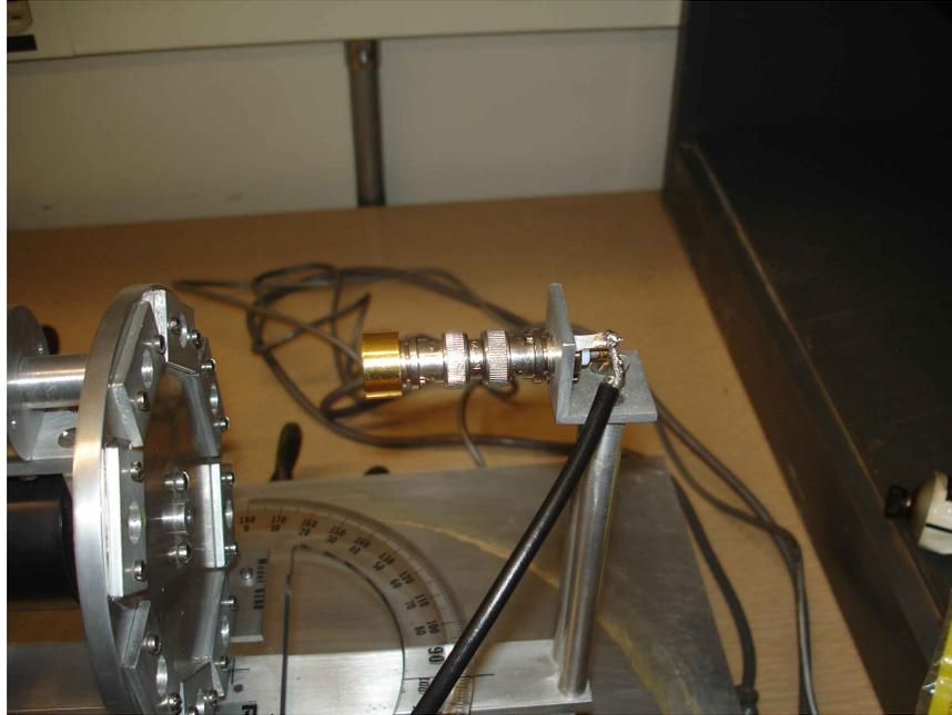
Figure 6.8: The sample wheel seen here is used to hold thin material films a few atoms thick in order to measure the deflection created by the nuclei of the atom. In addition the protractor is used in relation to the detector arm to determine the angle of deflection being measured.
