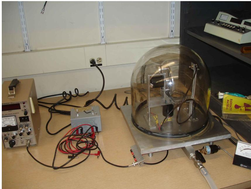
Figure 6.1: Full setup of the Rutherford Scattering Experiment. On the left there is a standard Ortec electronic counter. In the middle is the control box for the setup. There is a switch for rotating the sample wheel, and a switch for moving the detector through a range of angles.
