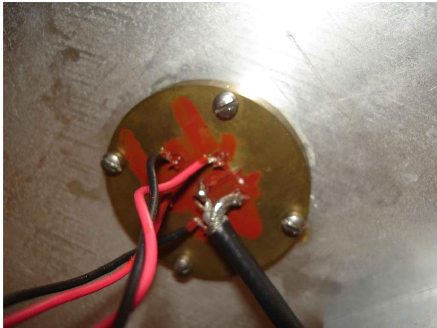
Figure 6.5: These connections are connected into the vacuum chamber through a contact plate on the under side seen here.
