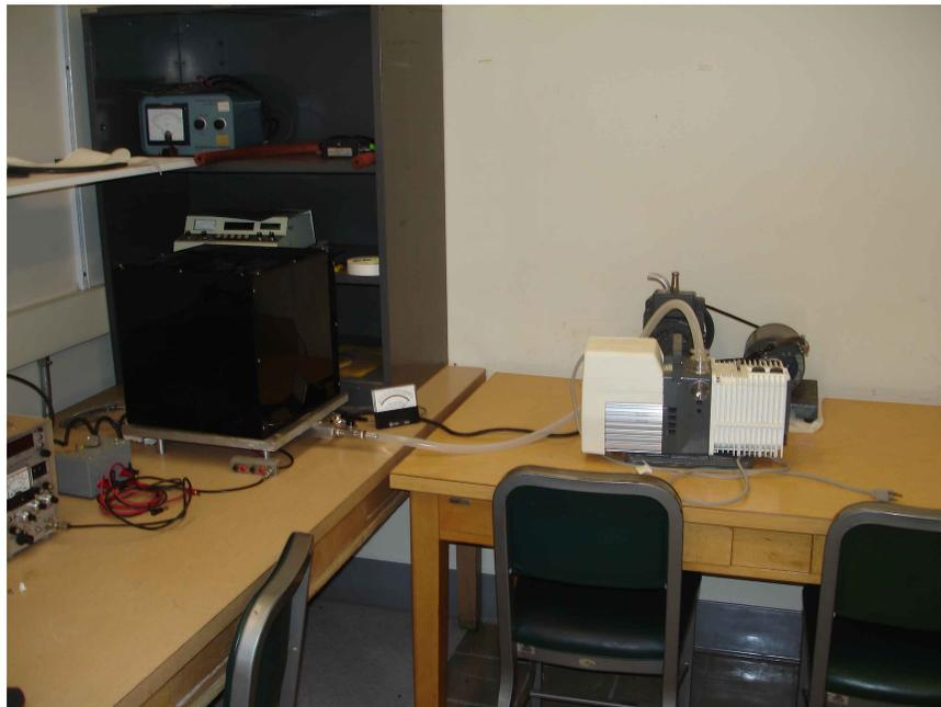
Figure 6.11: When the entire device is assembled a bell jar is placed over the detection devices, and a light dampening cover is placed on top of that. The setup is hooked to a vacuum pump and a vacuum is created in order to ensure that there are no loose particles floating around.
