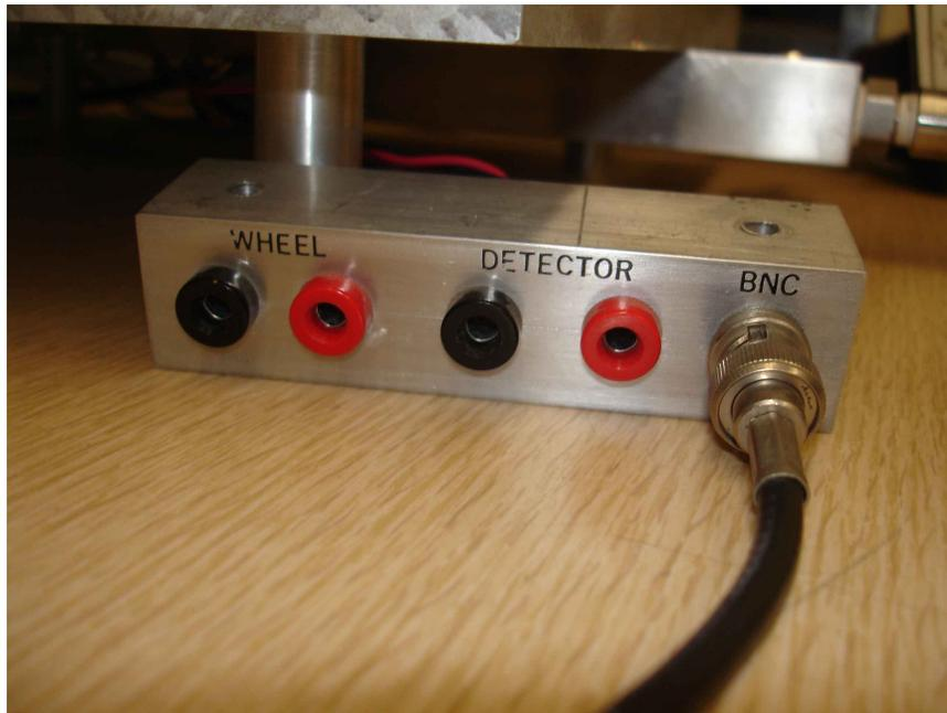
Figure 6.3: The counter and control box are connected to the main section of the experiment setup via cables into the following connector.
