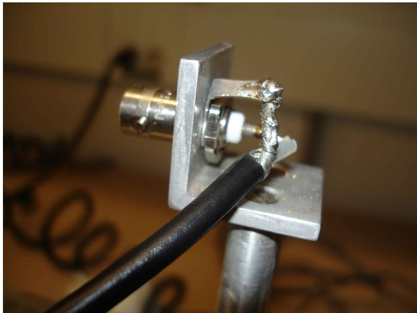
Figure 6.9: The detector connections were also re-soldered to ensure that they were working properly.
