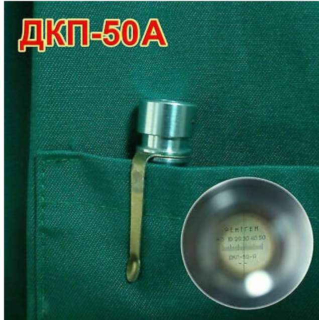
Figure 8 - Soviet radiation dosimeter. Source: URL
