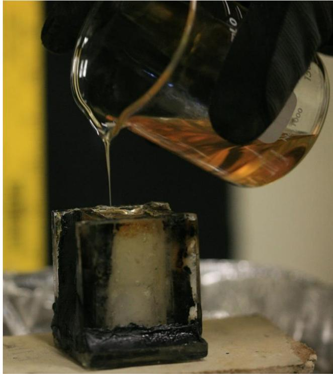
**Figure 3-6: Small container snow trial with ice block, snow, and oil**
