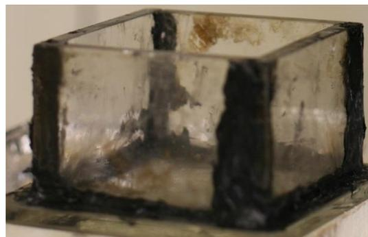
**Figure 3-3: Large container assembled using high temperature cement**
