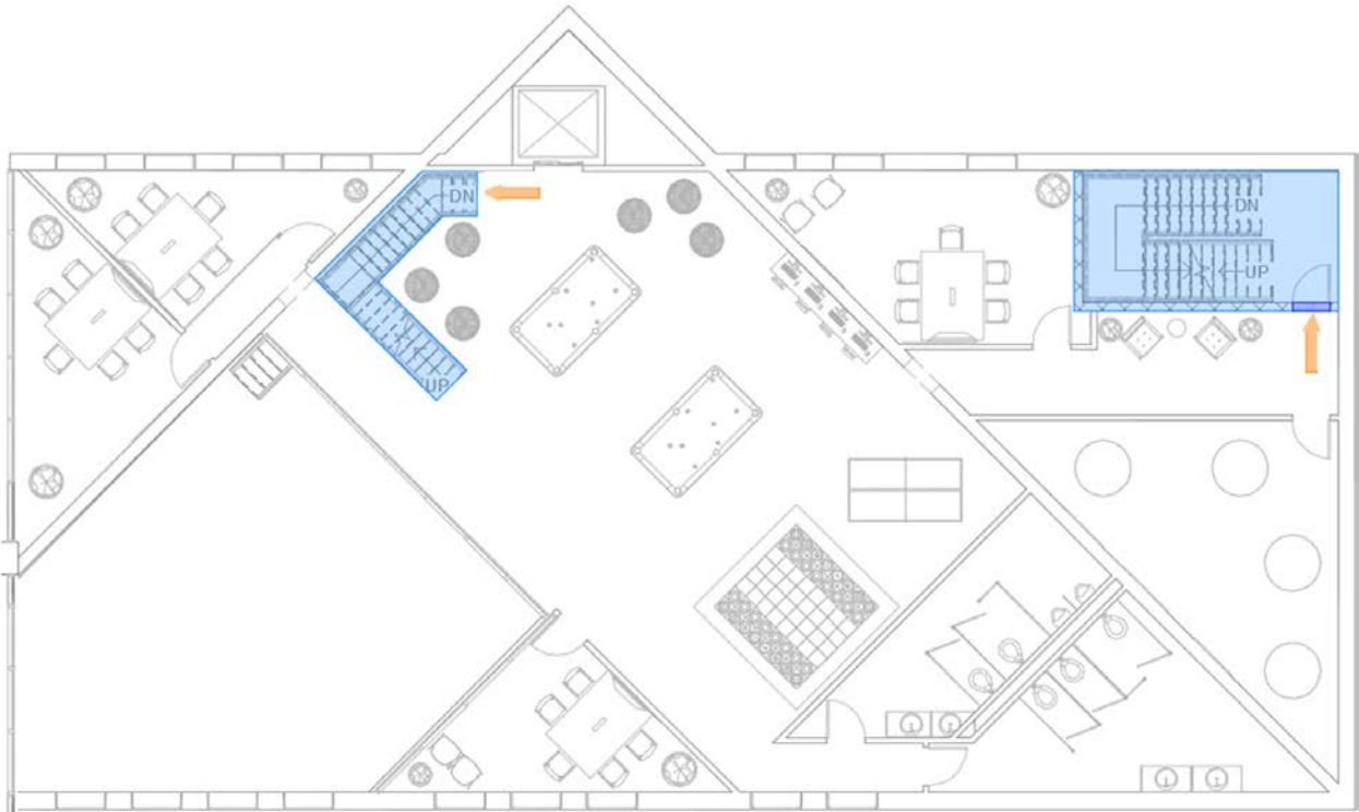
Figure 50: Student Building Second Floor Egress Plan
