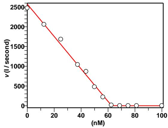
Figure 10. Inhibition curve for compound A with Q7K protease, gave a  $K_i$  of 0.001 nM.
