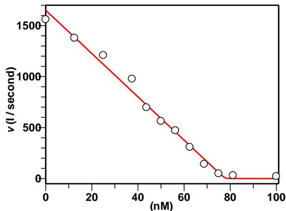
Figure 12. Inhibition curve for compound A with M1 mutant protease, gave a  $K_i$  of 0.001 nM.
