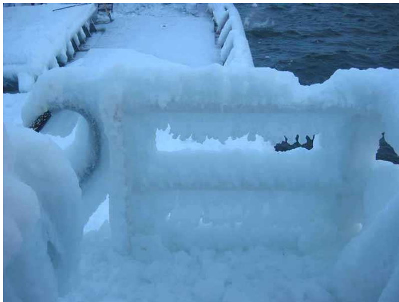
Figure 2-1: Moderate ice build up on the deck and railings of a vessel.
